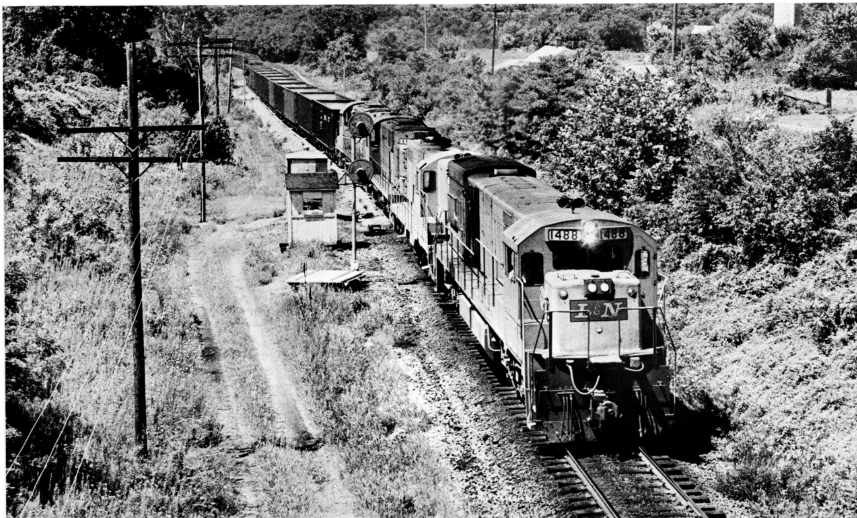
The installation of Centralized Traffic Control (CTC) on the old "KY" subdivision between Cincinnati and Corbin was completed in 1968. Where double track used to continue, U30C 1488 leads a southbound hopper extra through the high-speed turnout onto single track at Catawba, Ky. on a hot August 20, 1978. (Jill Oroszi)
