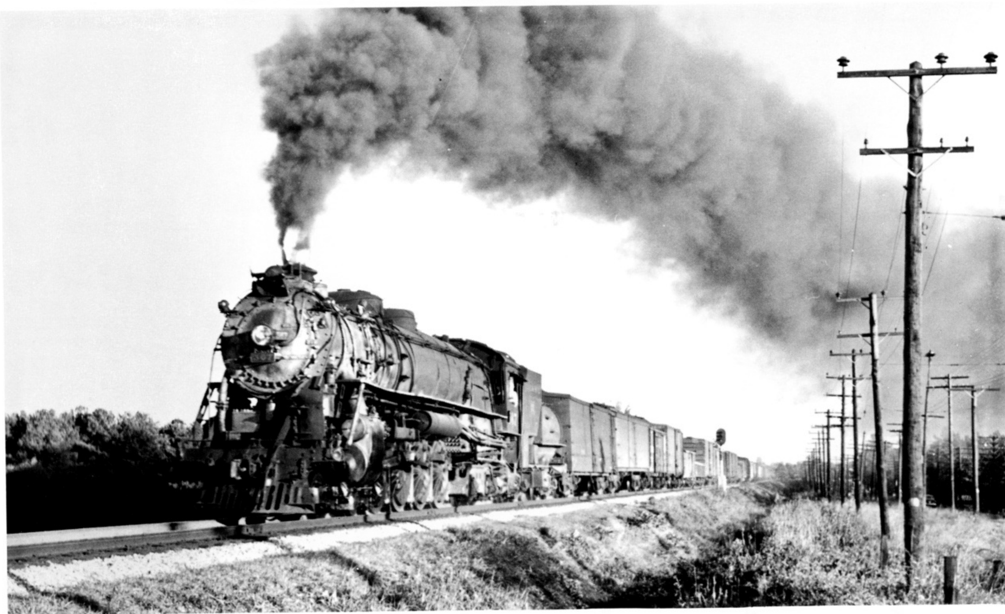
Nashville, Chattanooga & St. Louis "Dixie" No. 567 lays down sand as she accelerates a westbound manifest out of Smyrna, Georgia. The 567 was a member of the first five 4-8-4's delivered to the NC from American Locomotive in 1930. Lateral-motion boxes on the first two driving axles earned the fly-weight 4-8-4's their most enduring nickname--"Gliders." (R.D. Sharpless/F.E. Ardrey, Jr. Collection)
