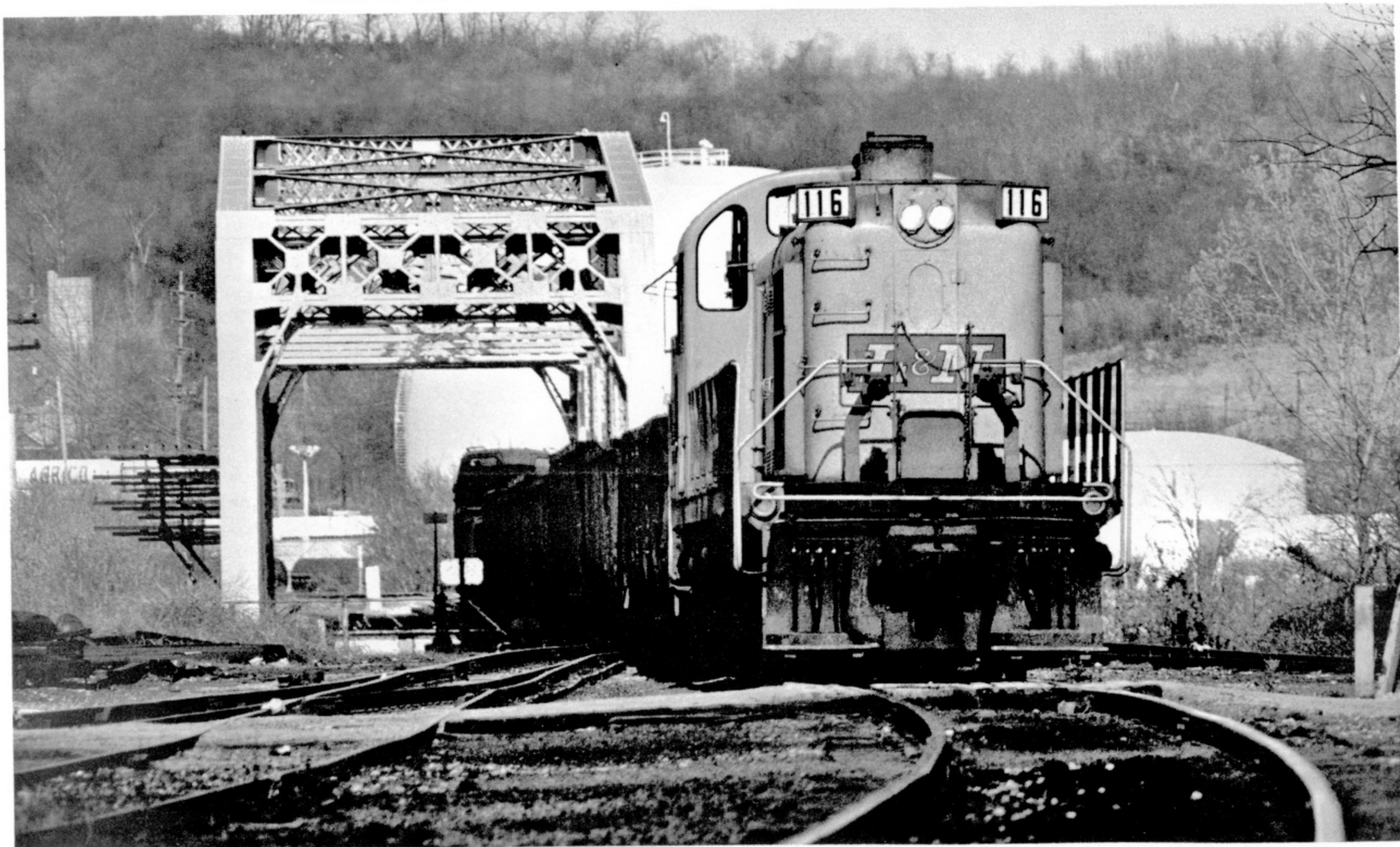
The versatile Alco RS3 was a familiar sight over most of the L&N. No. 116 from this distinguished fleet is shown in its final year of operation crossing the Licking River bridge in Covington, Ky. When this shot was made on April 13, 1974, the venerable engine had toiled almost 21 years for the L&N. An ex-Monon cab brings up the rear as the train heads for DeCoursey. (David Oroszi)
