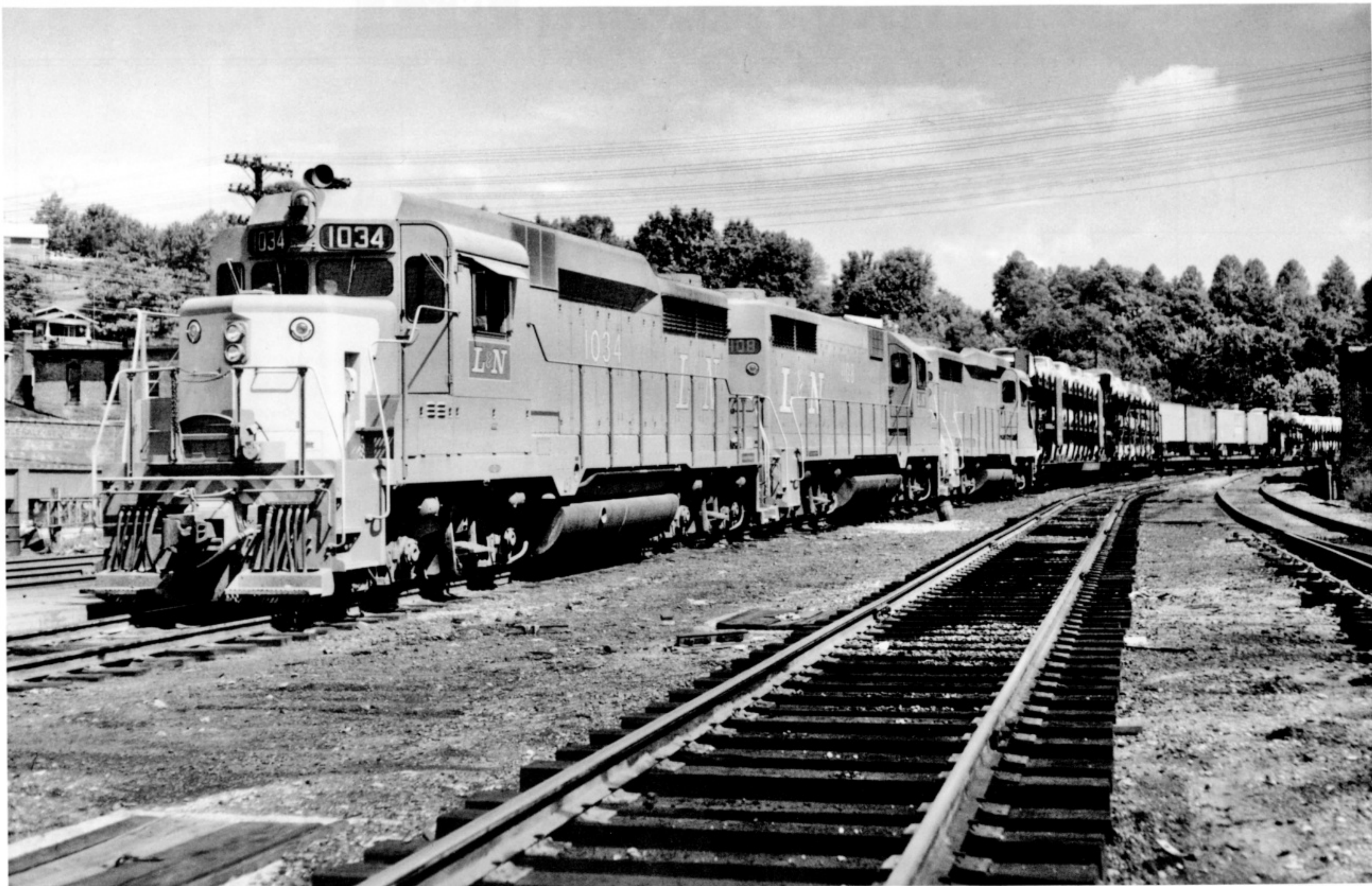
On July 15, 1964, tri-level automobile service on L&N's Cincinnati-Atlanta main is just months old. A clearance improvement project completed that year allowed the inauguration of this train, southbound "Autovan" No. 45, rolling up for a crew change at the Corbin, Kentucky passenger station. On the point, two GP30s are spliced by a new GP35. (Steve Patterson Photo)
