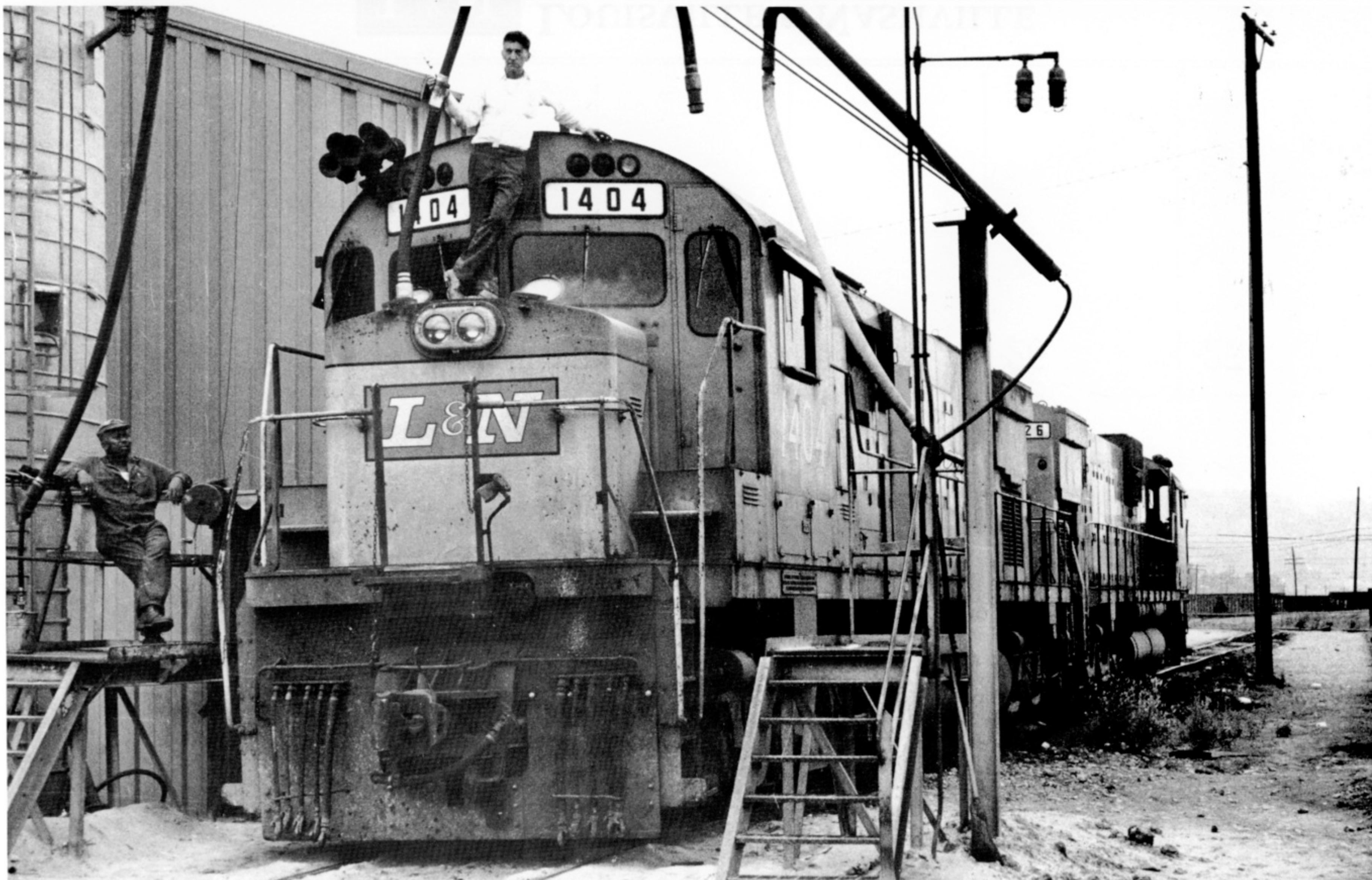
Two big Alco Centuries get a shot of “sea shore” at DeCoursey, Kentucky on June 17, 1973. The first unit is C628 No. 1404, part of a 12-unit order that ushered in the era of the six-motor unit on the L&N in 1964. The second unit is C630 No. 1426, added to the roster in 1966. The big Alcos were frequently found in coal train service on the eastern half of the L&N system. (Dave Oroszi Photo)
