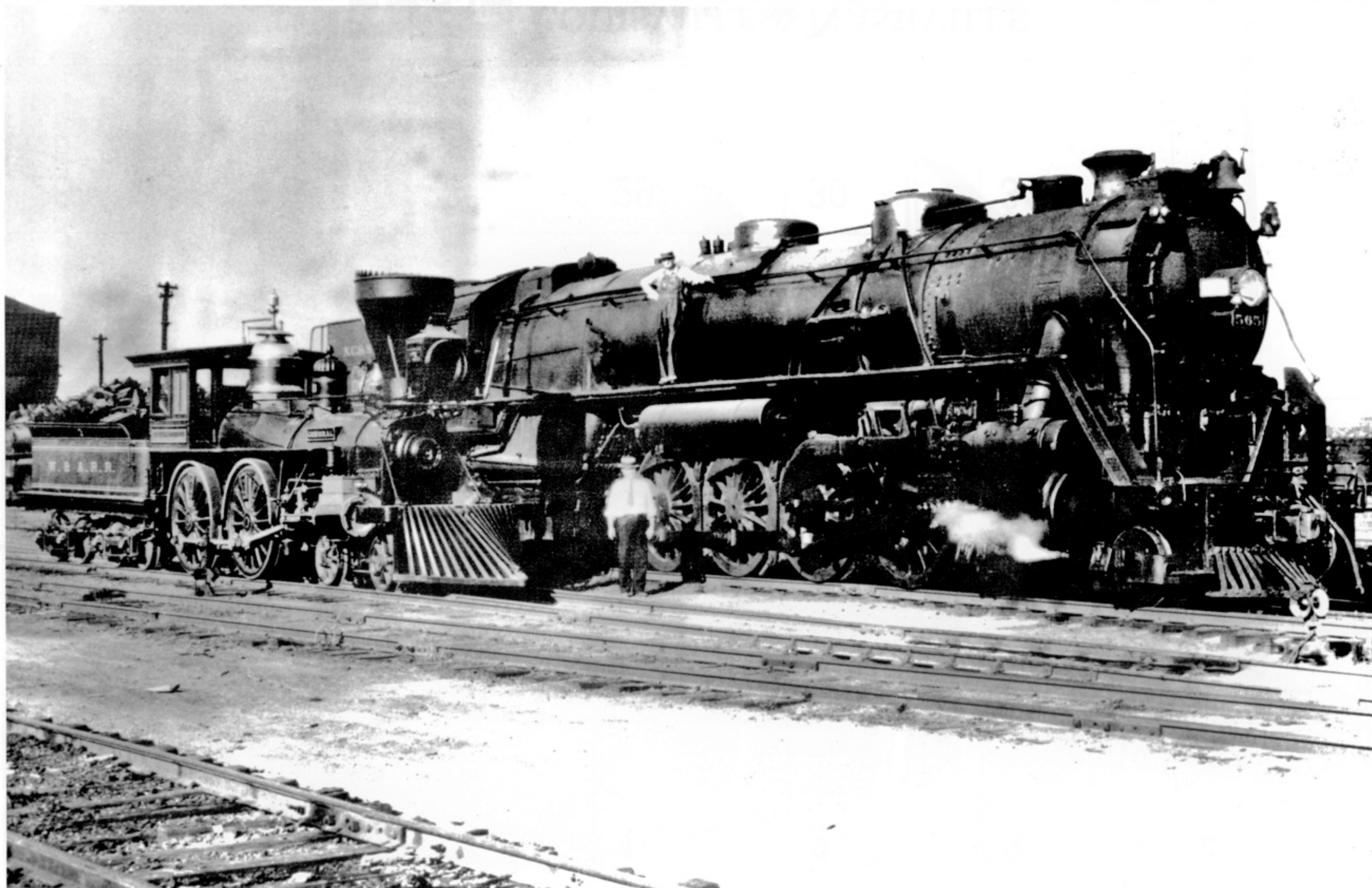
NC&StL "class" engine No. 565 is shown beside the famous Civil War General in this scene from the early '30s. The 4-8-4 was delivered to the Dixie Line in 1930 as the first of five such "Dixie" engines. NC enginemen quickly nicknamed them "Gliders," because of their lateral motion drivers. The "modern" 565 was scrapped in 1951, but the General was resteamed by the L&N in 1962, and today resides in a Kennesaw, Georgia museum. (L&N Collection/UofL Archives)
