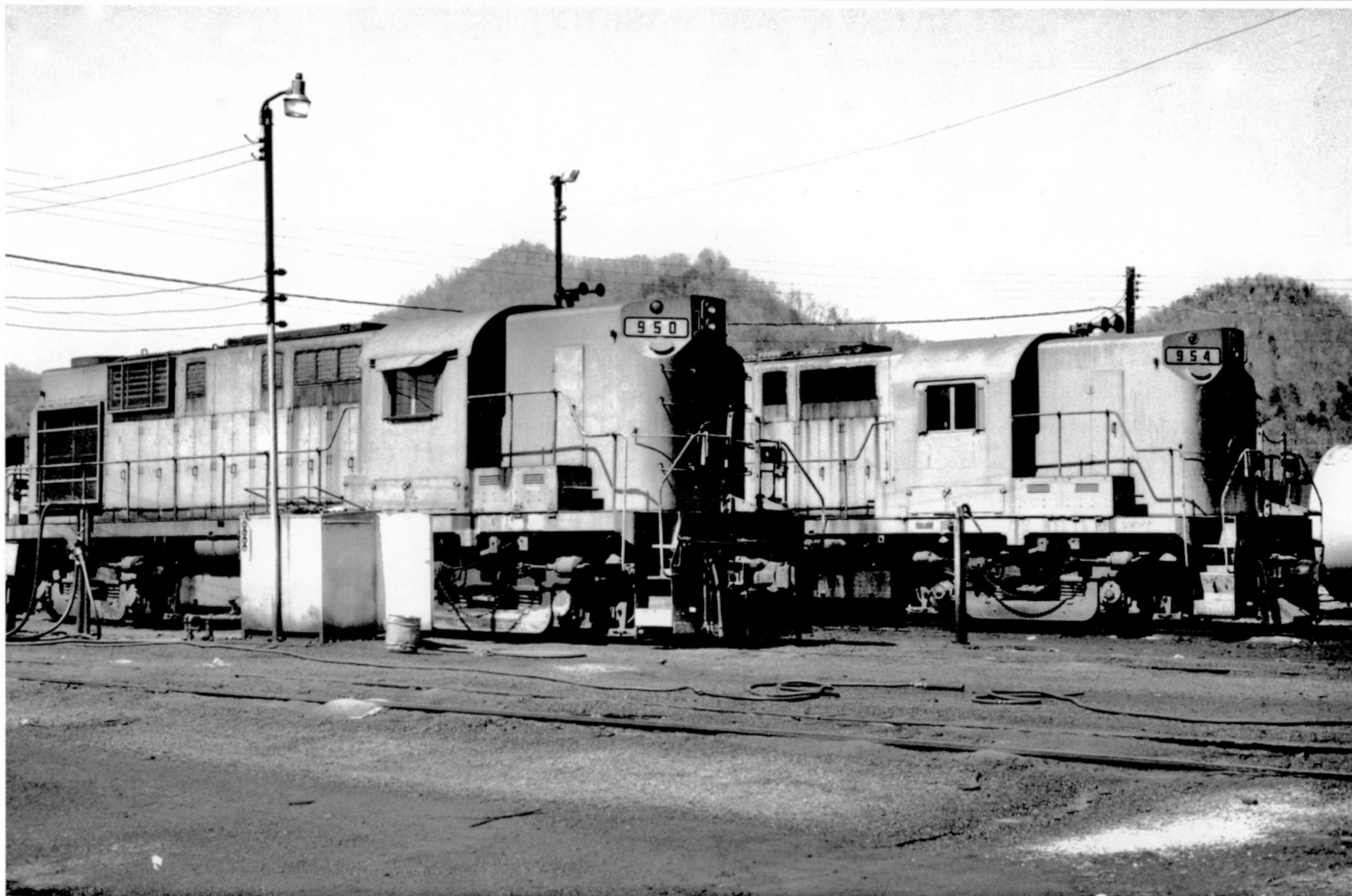
Two latter-day additions to L&N's Alco fleet rest their 251 prime movers at Ravenna, Kentucky in the late-'70s. The two RS11s initially came to Kentucky on lease from SCL in April 1976, but were acquired outright four months later. Part of a ten-unit group, these two were ex-SCL 1202 and 1206 respectively. (Dave Lichtenberg Photo)
