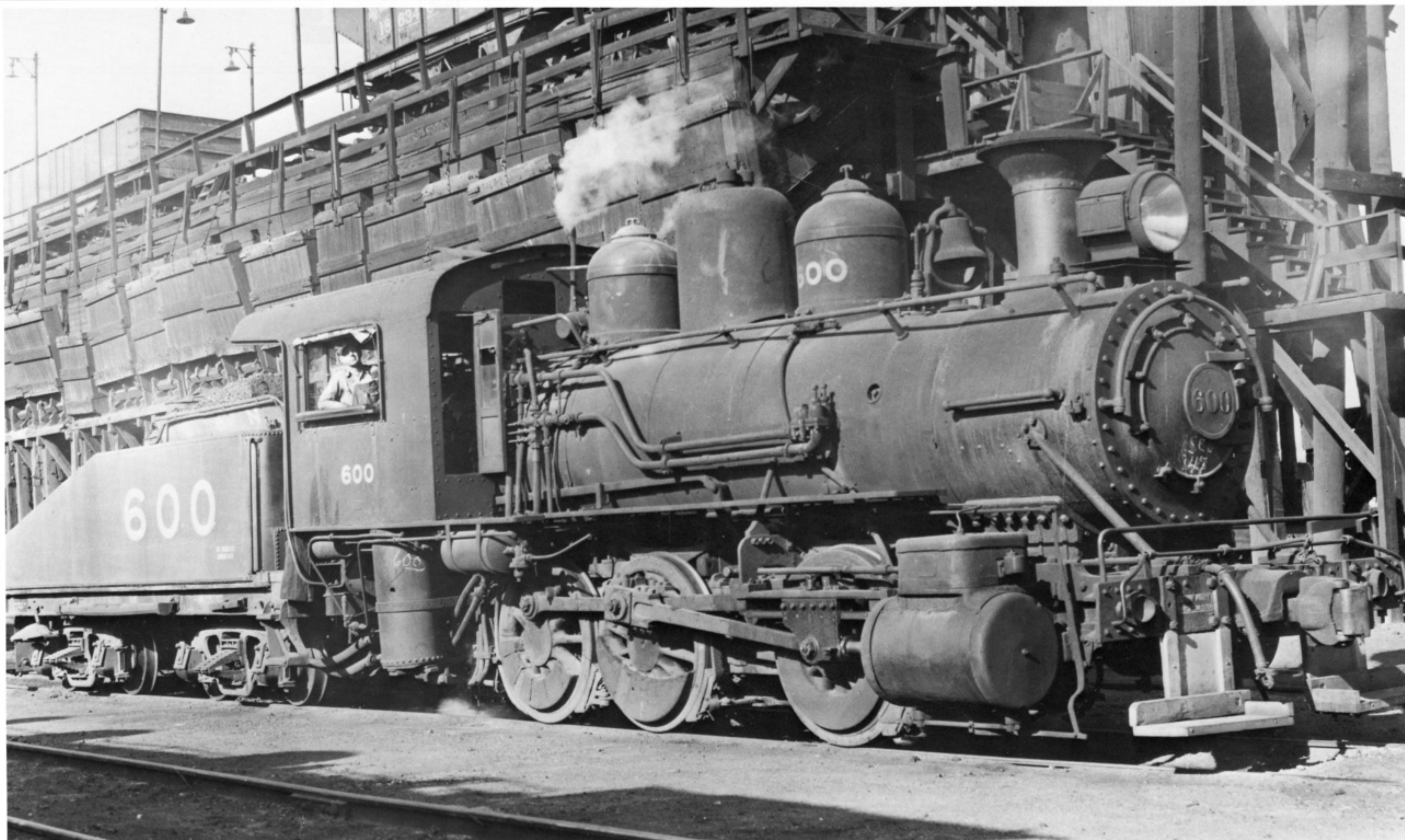
L&N managed to get an incredible amount of service from some of its steam locomotives. Case in point: B-6 no. 600 was rebuilt from an H-1 class Consolidation of the same number, built by Rogers in 1884. When the engine was retired about a year and a half after this April 6, 1947 photo at Birmingham's Boyles Yard, the engine rounded out nearly 64 years of service. Note the unusual spark arrestor on the engine's stack. (Frank E. Ardrey, Jr. Photo)
