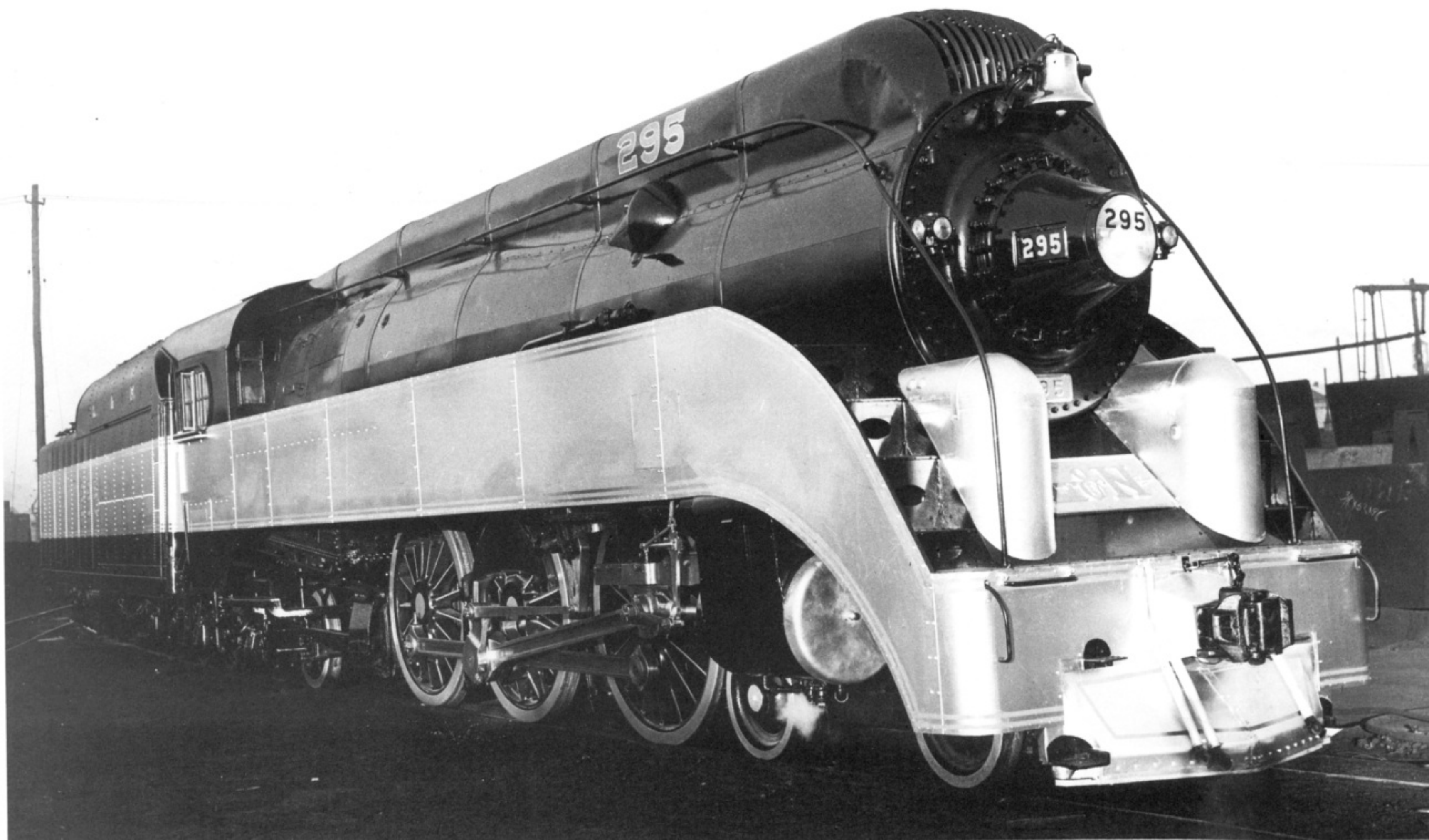
In the Fall of 1940, a very unique engine made its return to L&N rails, but in a very different garb, and with a very different mission. Former three-cylinder K7 Pacific 295, now converted to a two-cylinder engine, streamlined, and equipped with a custom-built 20,000 gallon, 27.5 ton tender, had just been unveiled at South Louisville. The 295 would soon begin handling the every-third day South Wind streamliner on L&N's portion of the run, Louisville-Montgomery. After the long and dreary years of the Great Depression, the 295 heralded new optimism for passenger service on the Old Reliable. (L&N Photo/UofL Archives)
