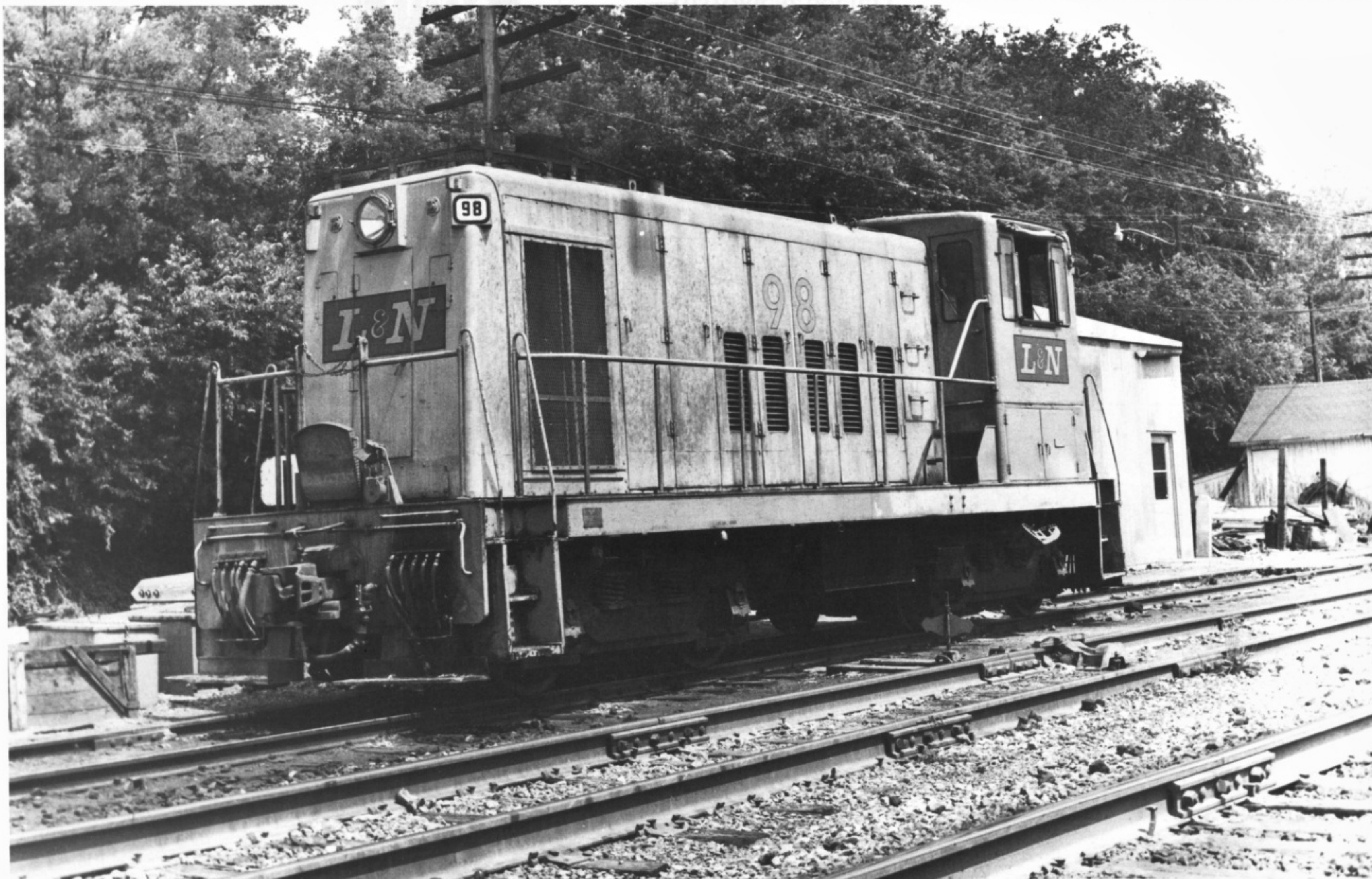
L&N class S3 GE 70-tonner 98 (one of two on the roster) was rebuilt at South Louisville in 1966 with an Alco 800 horsepower prime mover (200 more horsepower than the engine's original). The larger diesel engine required a raised hood. The system-unique was photographed at Gallatin, Tennessee, its normal operating base, in June 1969. (Bob Bell, Jr. Photo/J. Allen Hicks Collection)
