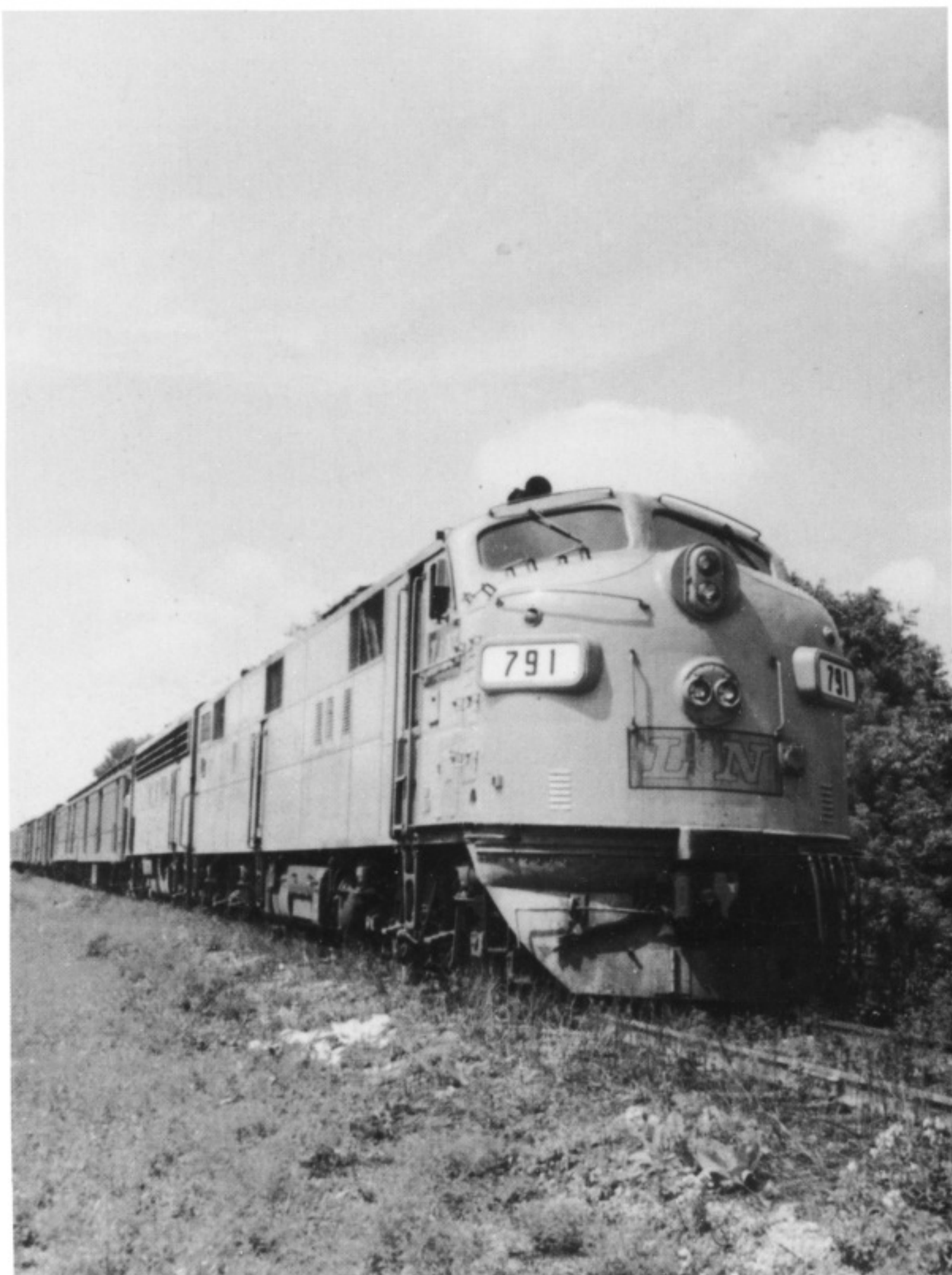
Train 4 is in the siding at Campbellsburg, Kentucky in September 1966 to meet the southbound Pan-American . E7 791 was the recipient of a South Louisville "beauty treatment," with external Gyalight above and sealed beam headlight below. (Charles B. Castner, Jr. Photo)
