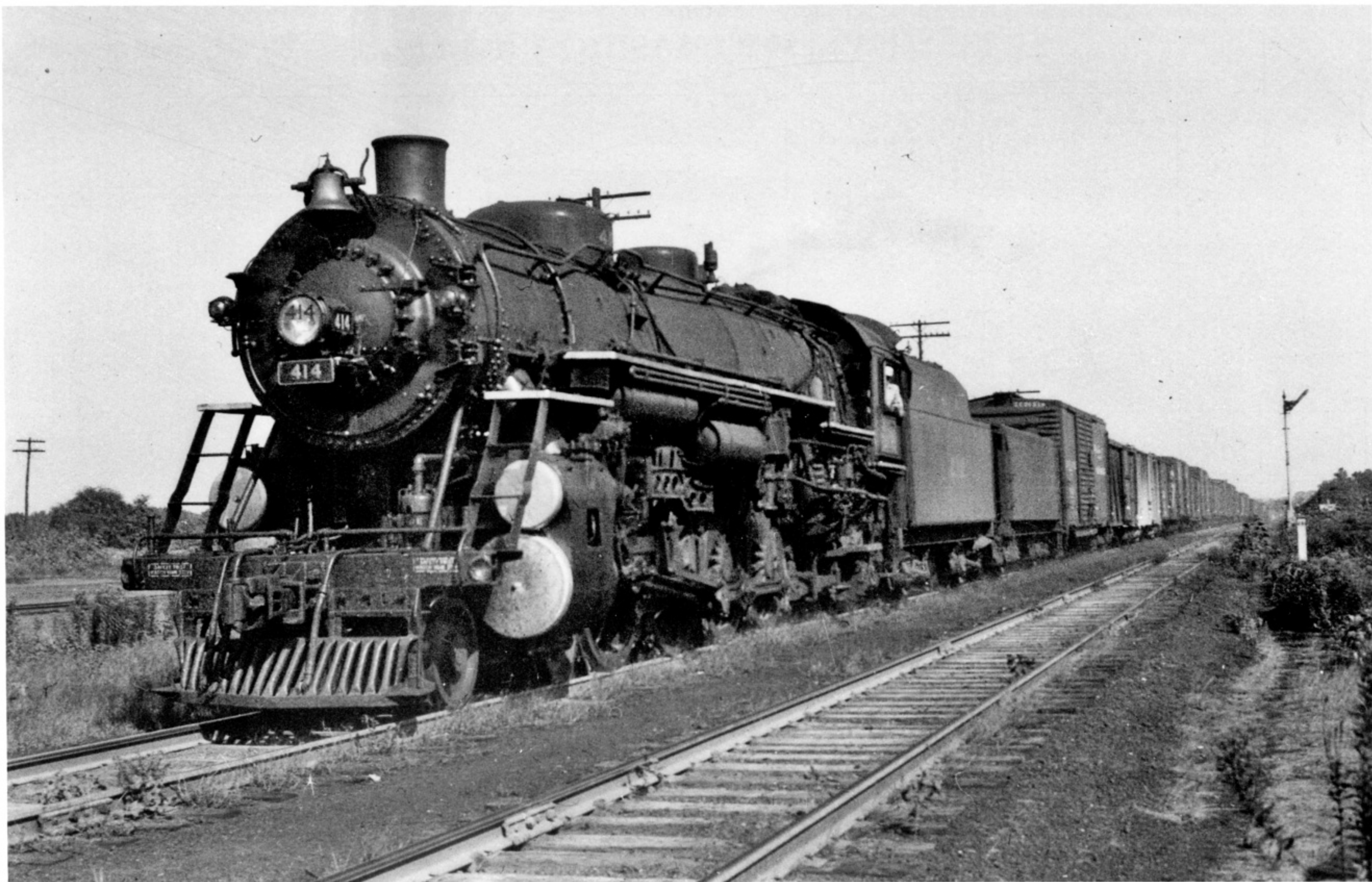
L-1 Mountain 414 was still looking sharp, with silvered cylinder head covers and running board edges, when photographed on a fast freight around 1950 at an unknown location. Note the auxiliary water tender, added to increase the operating range of the handsome USRA-design 4-8-2. (Ron Flanary Collection)
