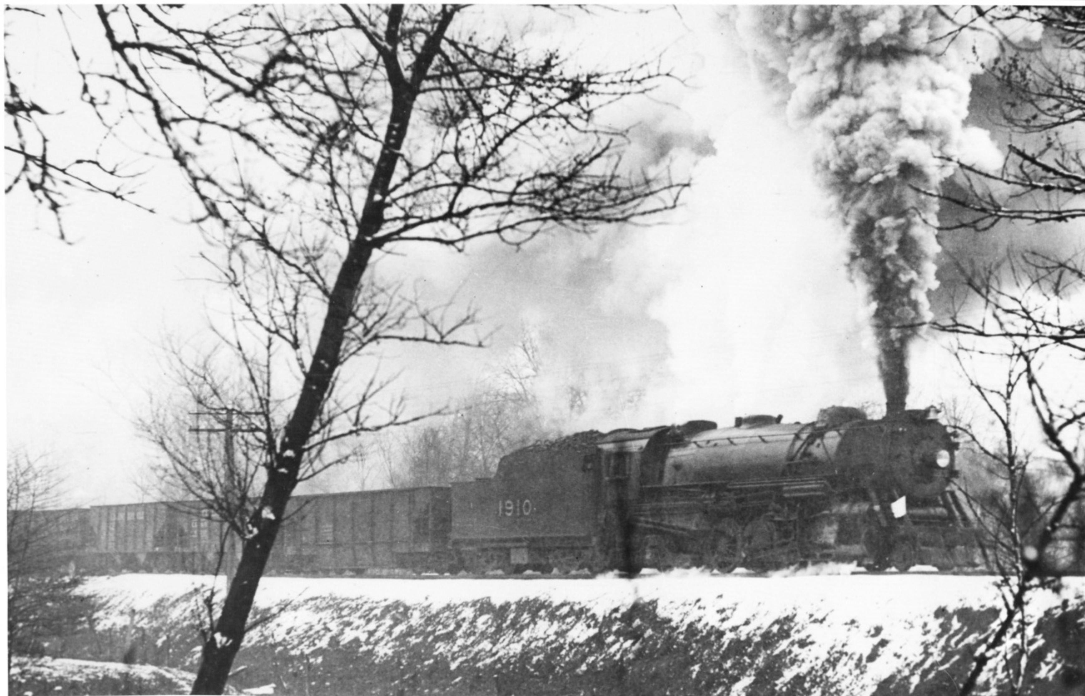
Falling snow begins to cover the countryside in northern Kentucky as a hopper train pounds by on the Kentucky Division main behind J4A 1910. This scene was photographed in the mid-'30s just south of DeCoursey. Note the white "extra" flags mounted on the pilot beam, rather than on the front of the smokebox above the classification lamps, as was later practice . (Ed Kuhr Collection, from Dan Finrock)
