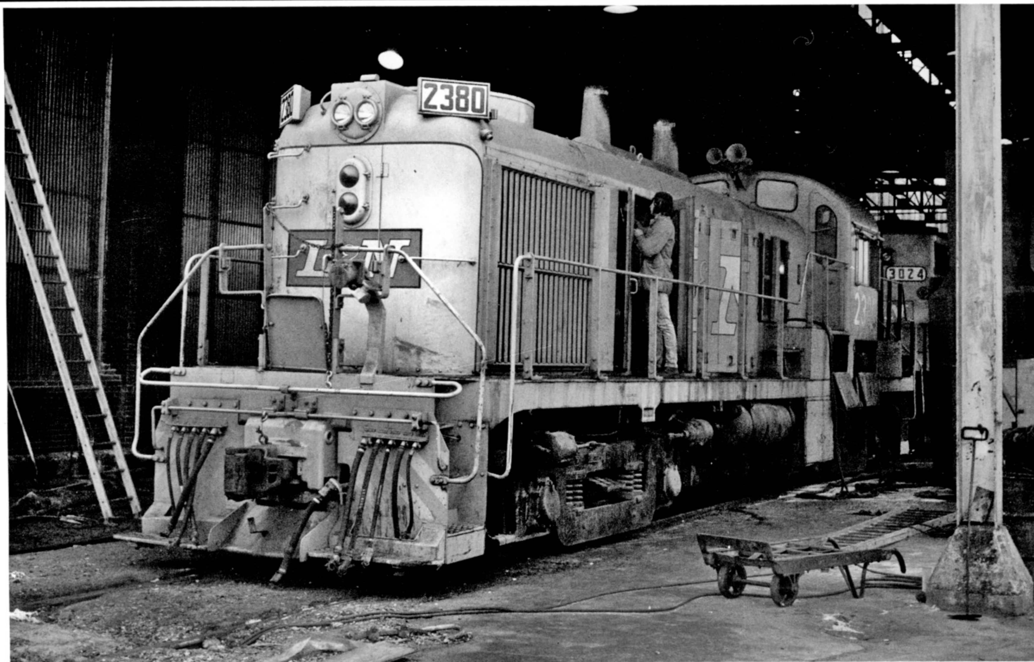
Alco RS3 138 was rebuilt at South Louisville in June 1969 with an EMD 567-C 1200 horsepower prime mover, and redesignated an RS3m. On November 2, 1972, it was renumbered to 2380. Just over a month later, the hybrid unit was receiving attention at the shop. (L&N Photo/L&NHS Collection)
