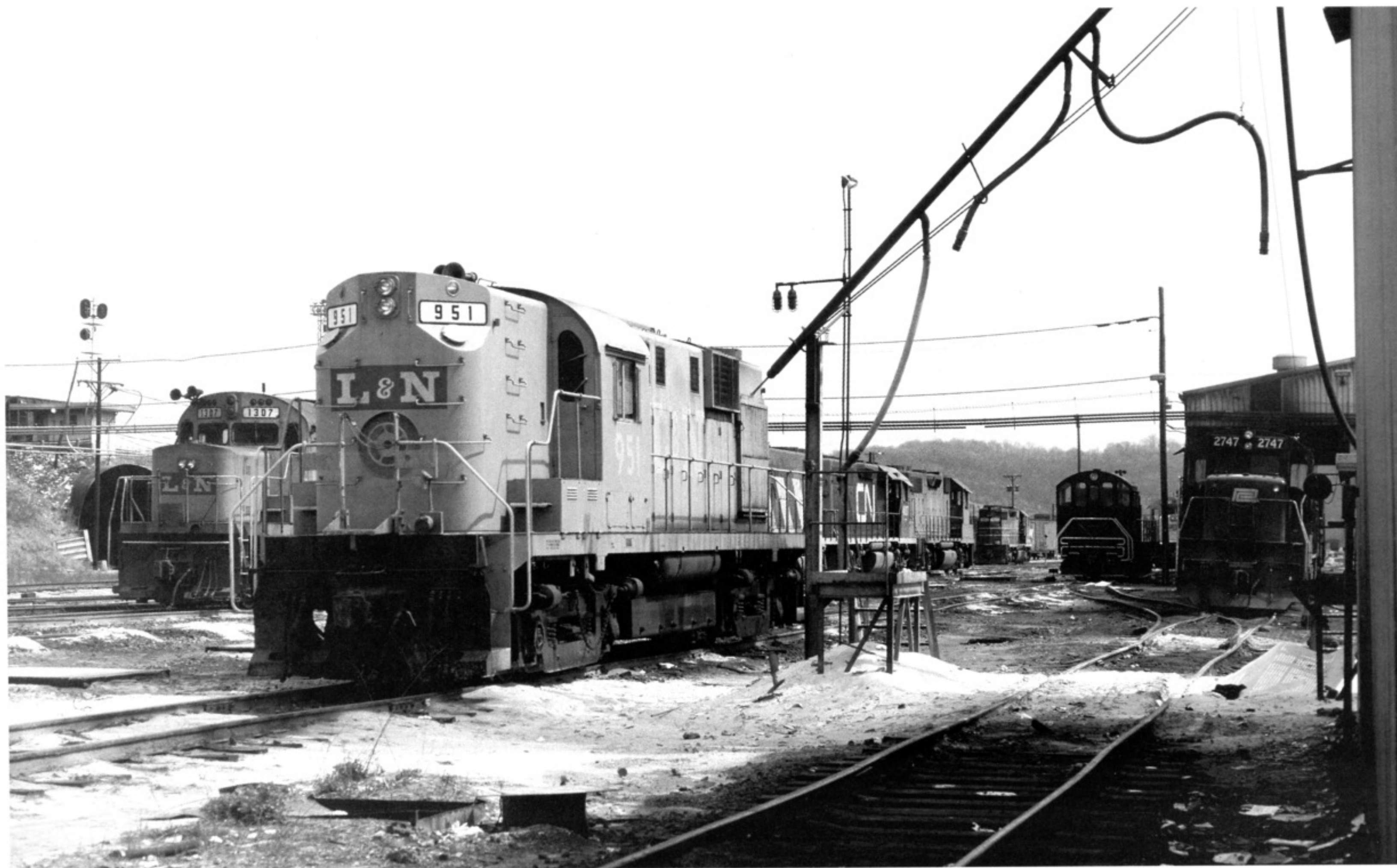
Typical of the mid to late '70s on the L&N is this eclectic group of motive power at DeCoursey on April 3, 1977. Prominent is Alco RS11 951 (an ex-Seaboard Air Line engine – number 101 – constructed in 1960), but also visible are leased/pooled units of Canadian National and Penn Central. (Mike Leach Photo)
