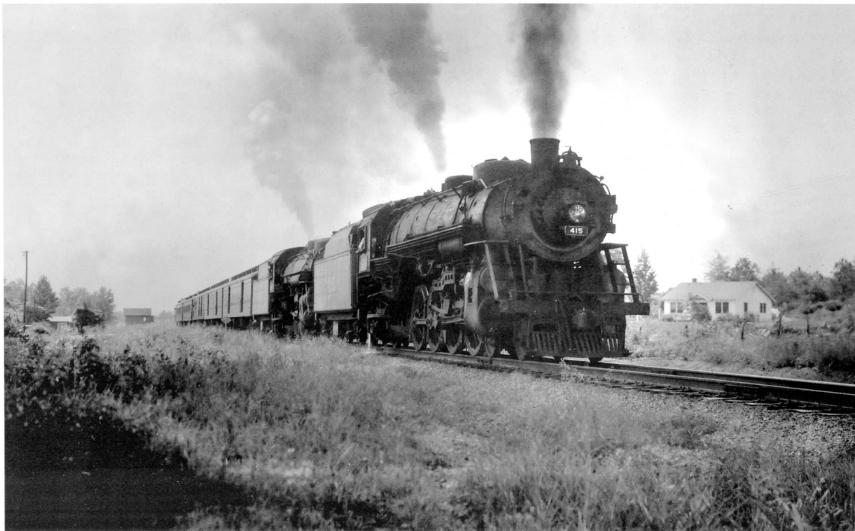
Near Birmingham in 1947, the safety valves on both L1 415 and K5 247 lift momentarily at a rural flag stop. This obviously overpowered passenger local would normally have a single 4-6-2, but the Mountain up front is being moved to balance power. (Gary D. Rolih Collection)
