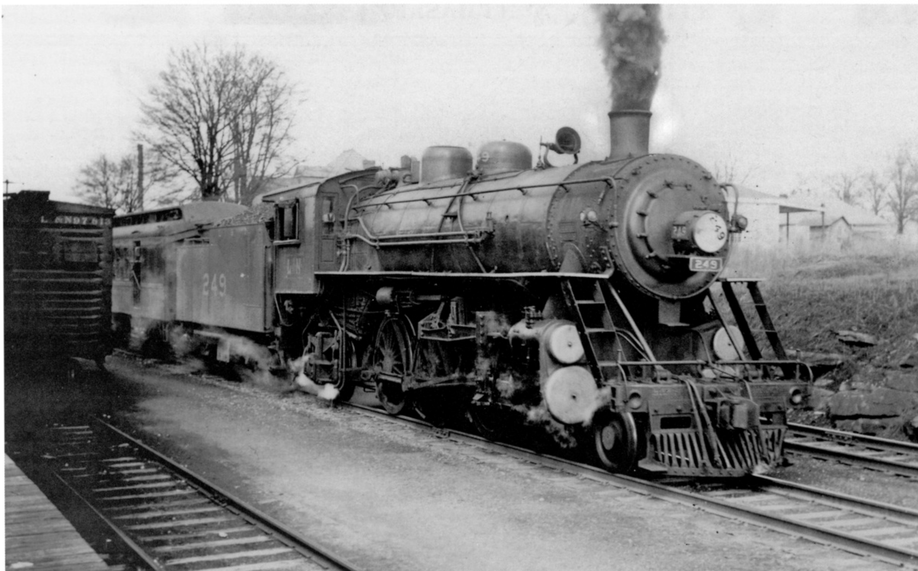
At Hartselle, Alabama on March 16, 1941, K4B Pacific 249 — its headlight lens askew — gets underway again after a brief stop with a passenger train. The 18 engines of this class were the last passenger engines constructed in L&N's own South Louisville Shops in 1920 to 1922. (Ron Flanary Collection)
