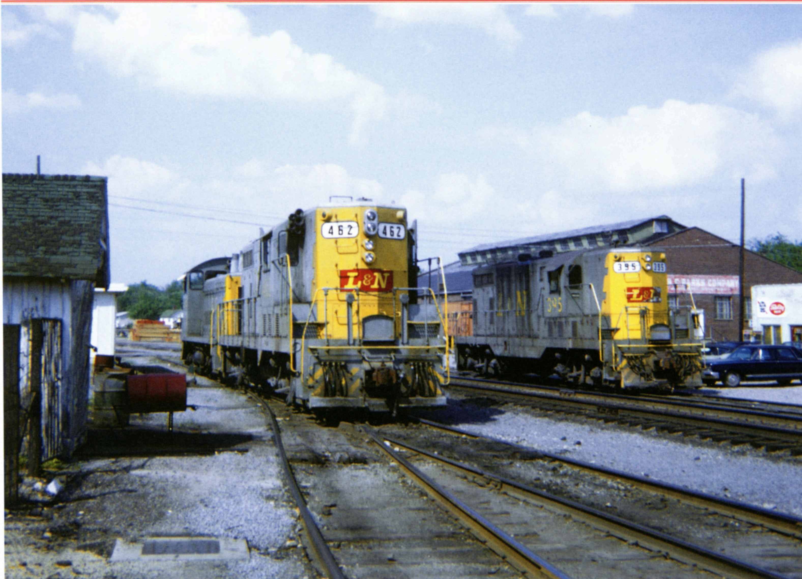
L&N GP7s 462 and 395 and a lone switcher are parked at the engine facility in Gallatin, Tennessee, in May 1971. While the 395 is an L&N original, the 462 was built in 1951 as NC&StL 1725. The unusual placement of the air horns on the engineer's side of the front hood for clearance purposes must have been an ear-splitting experience for the crew. — J. Allen Hicks photo
