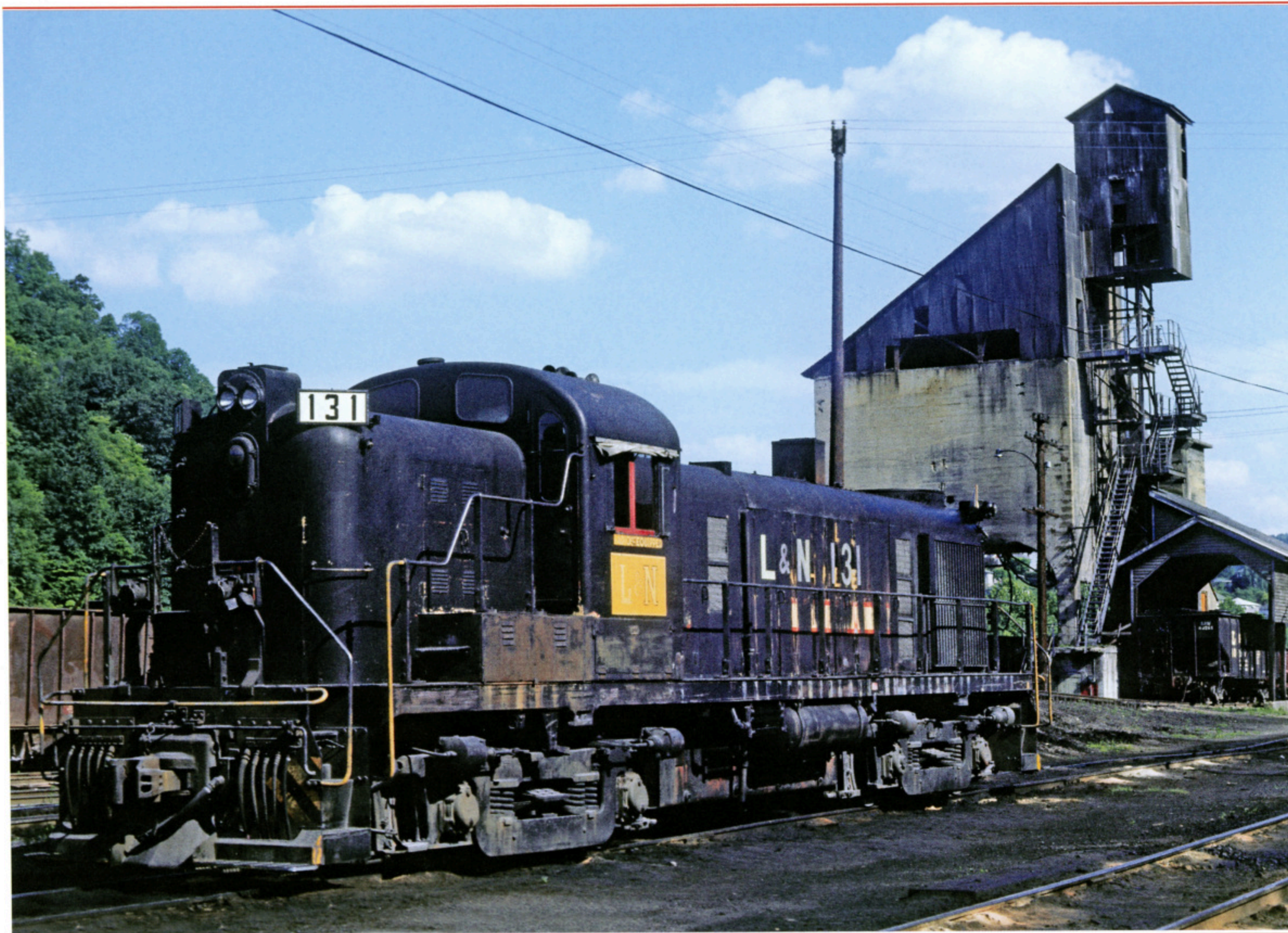
L&N Black RS-3 131 is parked in Hazard, Kentucky, in June 1969 with the impressive coaling dock in the background. The 131 was one of those RS-3s that somehow kept her original number to the end. It was subsequently cut down and recycled as a booster/slug in 1971, becoming the 2054. — Jim Boyd photo
