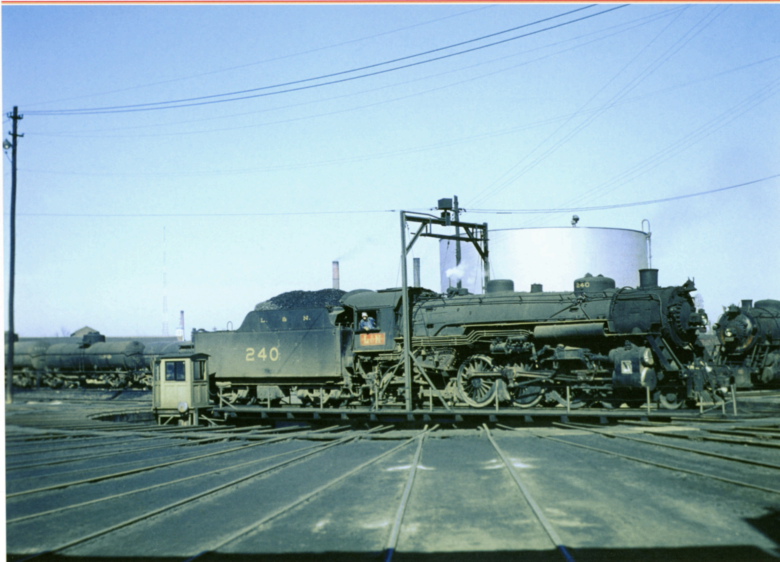
Classy 4-6-2 240 takes a spin on the turntable in South Louisville in the early 1950s. The 240 was built by Alco's Richmond Works in 1919 — the first of six light USRA Pacifics assigned by the USRA to the L&N. The K-5 class was considered one of the best overall mechanical and operating passenger engines on the L&N, which acquired 26 such engines. The 240 itself was consigned to scrap in 1953. —Jack Fravert photo
