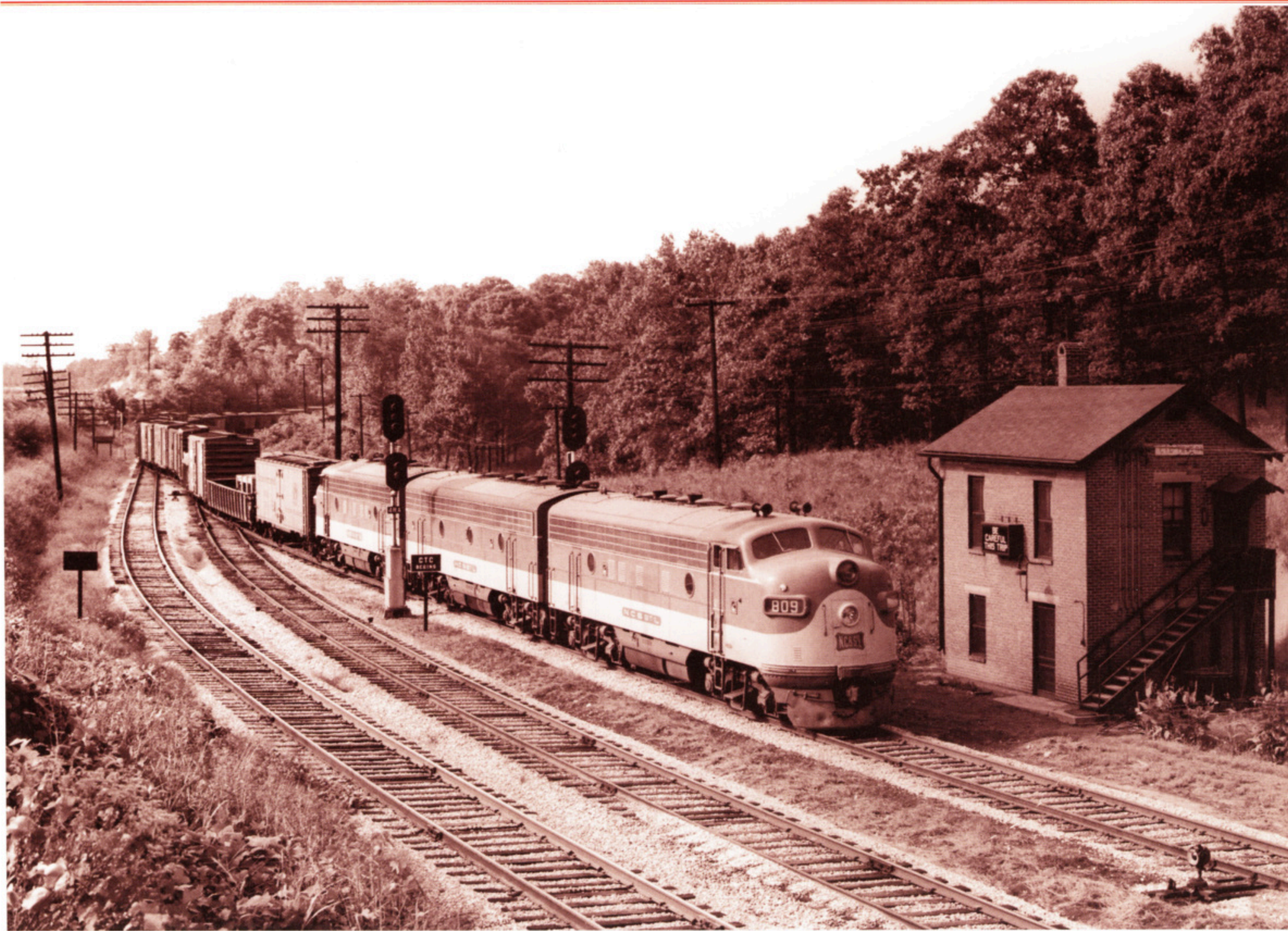
L&N In June 1951 EMD F7 809 is on the point of an A-B-A F-unit set entering Hills Park Yard in Atlanta. NC&StL's F-units were purely dual purpose power, working both freights and passenger runs. The B-units had steam generators for the latter work, while the A-units did not. — R.D. Sharples photo, F.E. Ardrey collection
