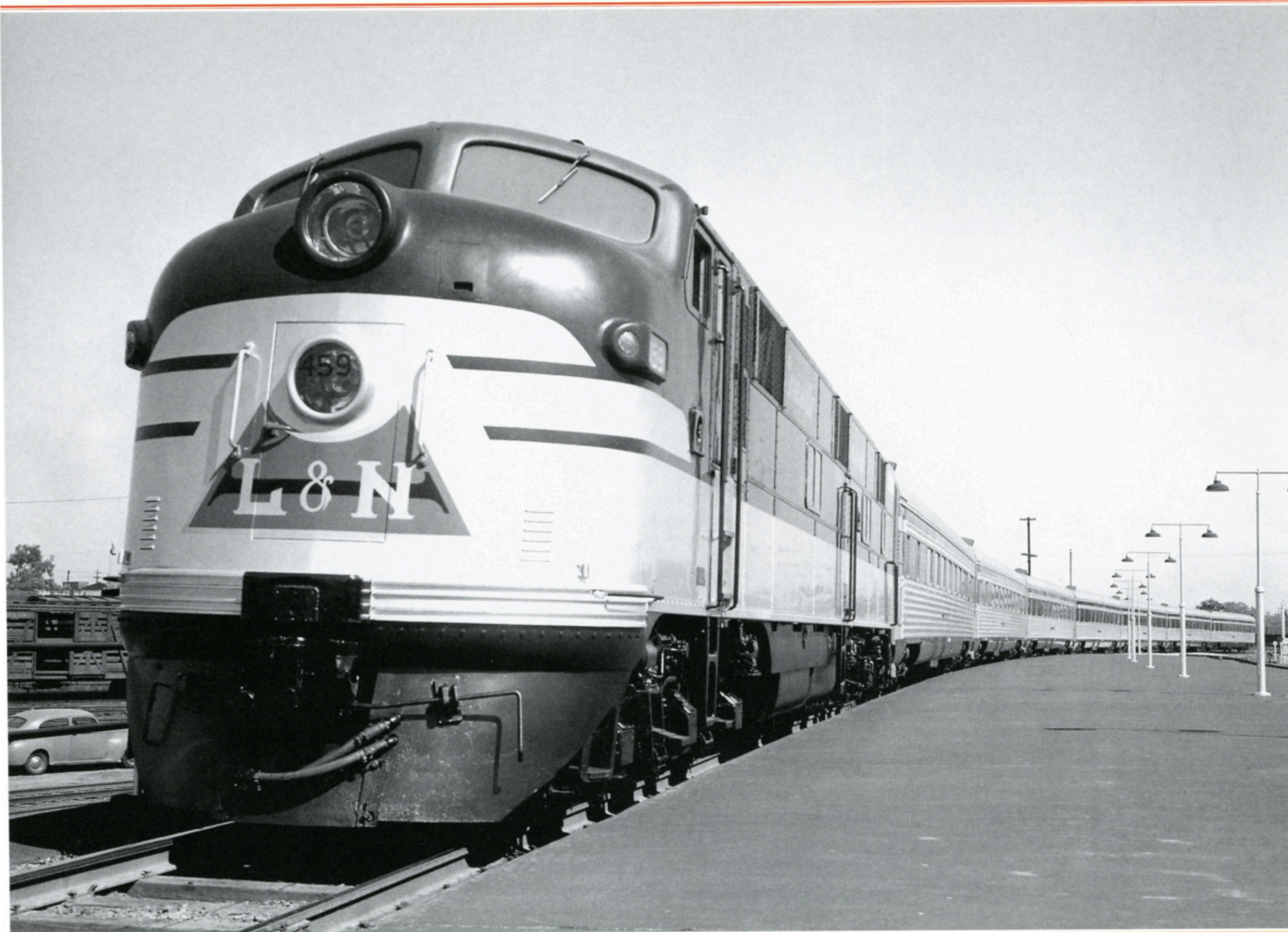
L&N In a classic publicity pose, EMD E7 759 powers the Humming Bird at the Baxter Avenue Station in Louisville, Kentucky, in November 1946. This is a pre-inaugural photo special heading south. The E7, dressed sharply in blue and silver, was 459A. All the E-units would soon be renumbered into the 750-series. —Kevin EuDaly collection
