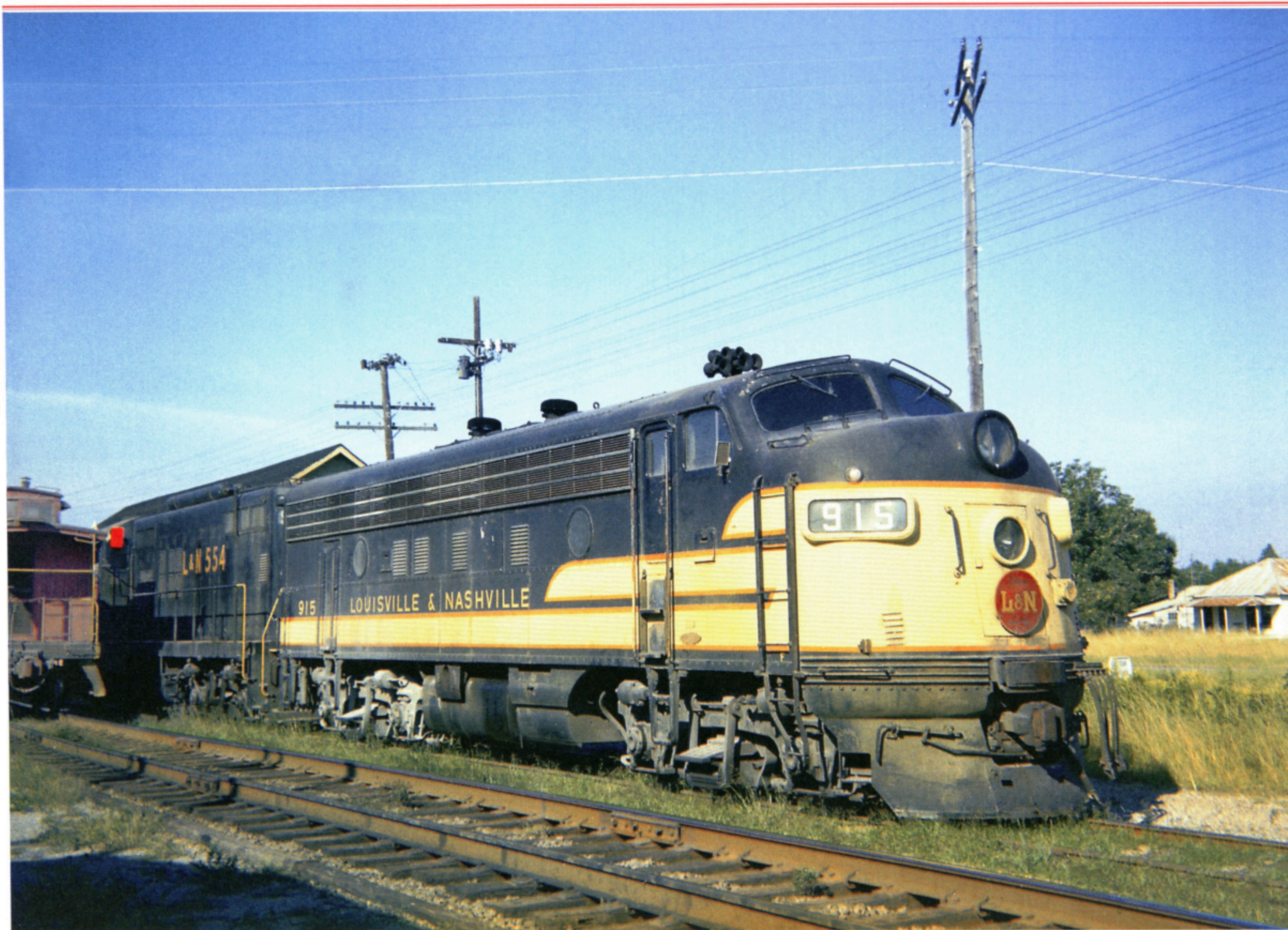
L&N On August 24, 1962, F-unit 915 is on No. 43 in the house track awaiting instructions at Kreole, Mississippi. The 915 was one of the last units to get the classic black and cream paint scheme. The metal medallion on the front replaced the painted triangular herald. The reflective marker on the caboose is also a recent change — replacing the kerosene marker lamps about this time.— J.G. Lachausse photo
