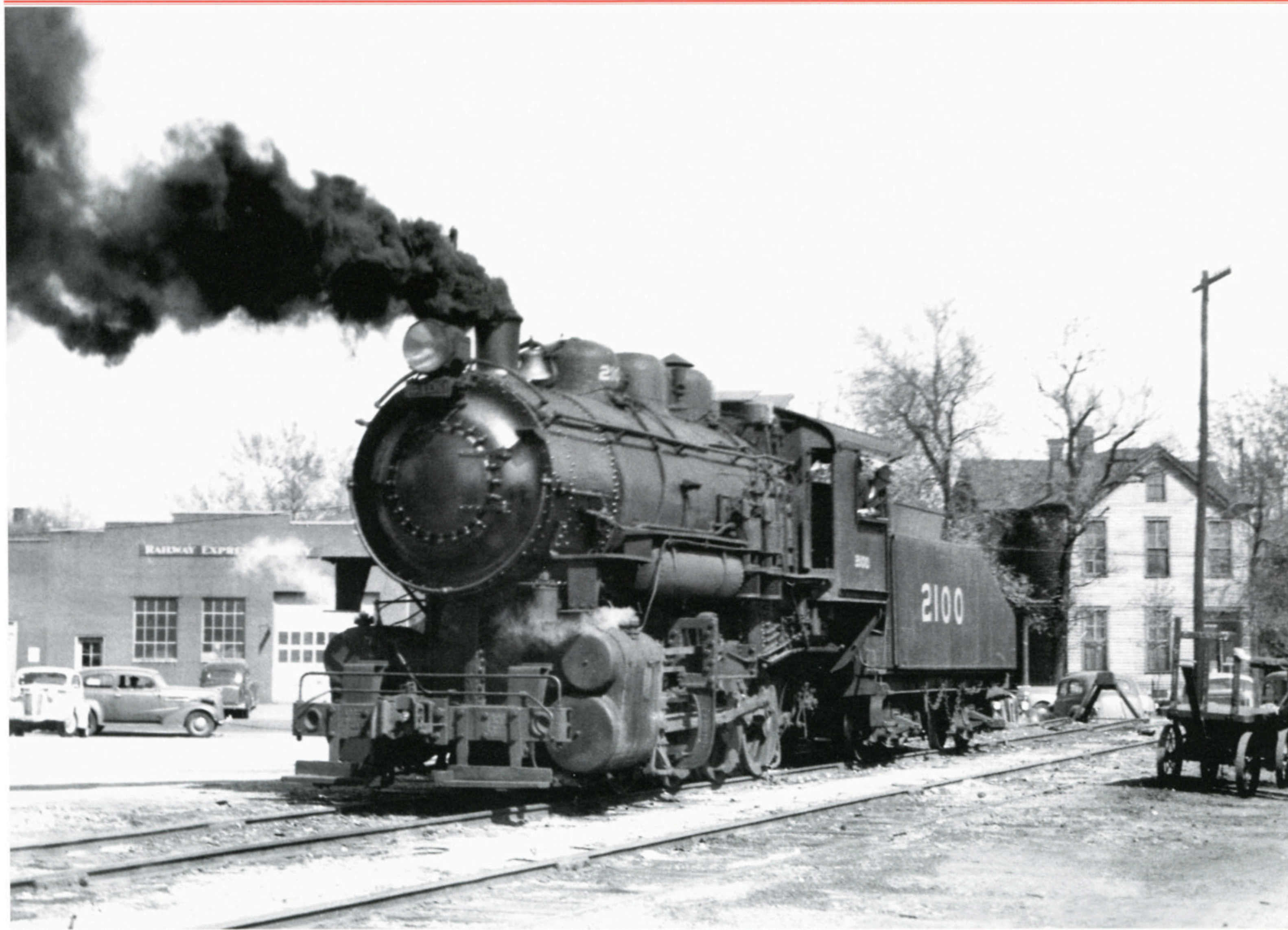
L&N Class C-1 2100 is under steam and smoking away in Evansville, Indiana, in 1949. The 2100 was built by the L&N at South Louisville Shops in 1915 and retired in 1952. This might be a smoke abatement demonstration. During the 1940s the L&N used different variations of over-fire air jets on the firebox to help reduce smoke on yard and switching locomotives working in urban areas. —Kevin EuDaly collection
