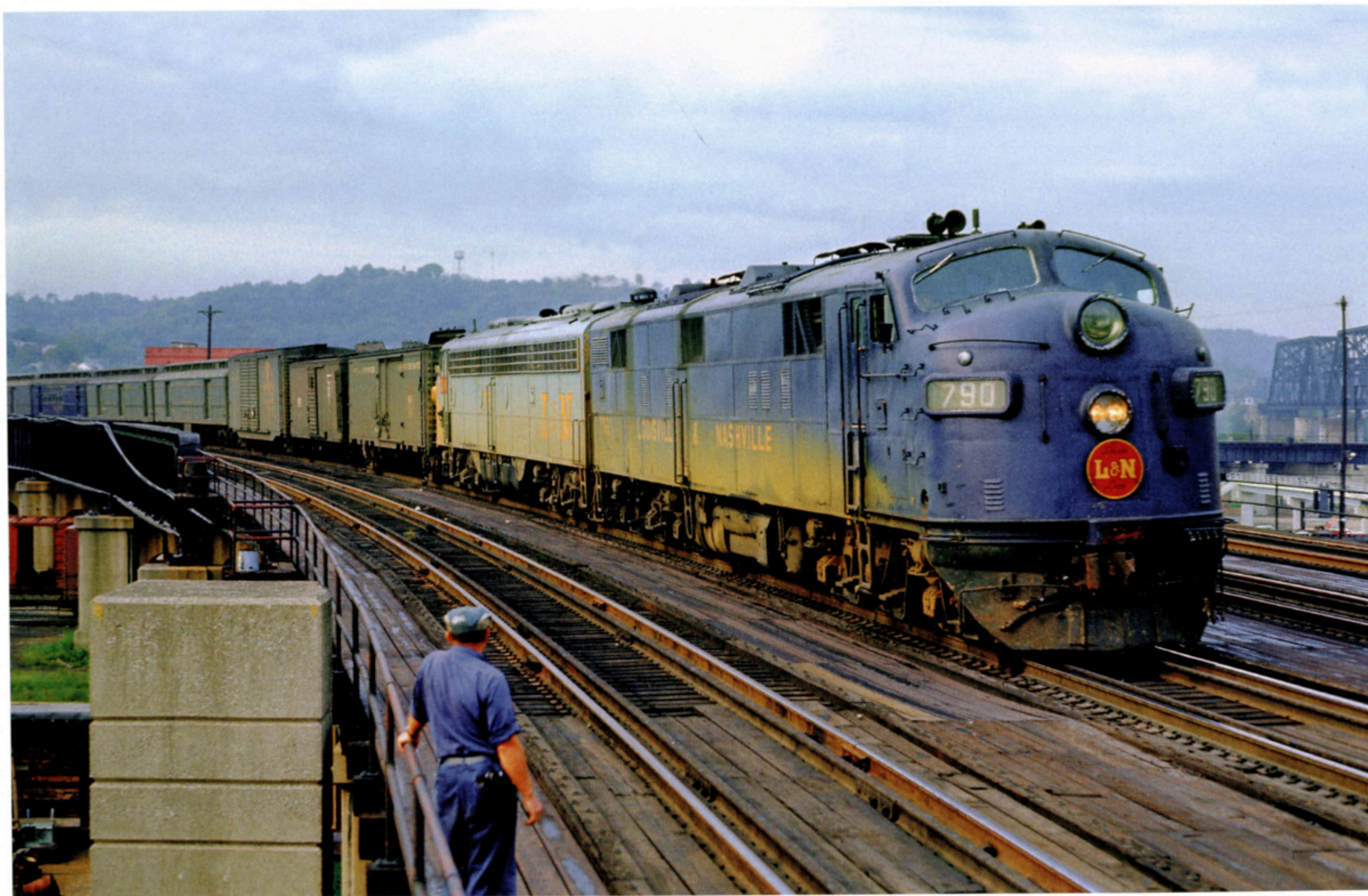
Although it was billed as a "Coach-Pullman Streamliner," this September 1965 Cincinnati scene of train 6, the northbound Humming Bird , hardly meets that description. Behind E7 790 and E8 797 is a train that includes at least seven head end cars — an empty REA express reefer, both a Pennsy and a Santa Fe express box, and four L&N cars, including an RPO. The train is curving off the viaduct connecting the C&O bridge with the south throat of Cincinnati Union Terminal. The black truss bridge in the right background is Southern's Cincinnati-owned CNO&TP double track span over the Ohio River. —Jim Boyd photo
