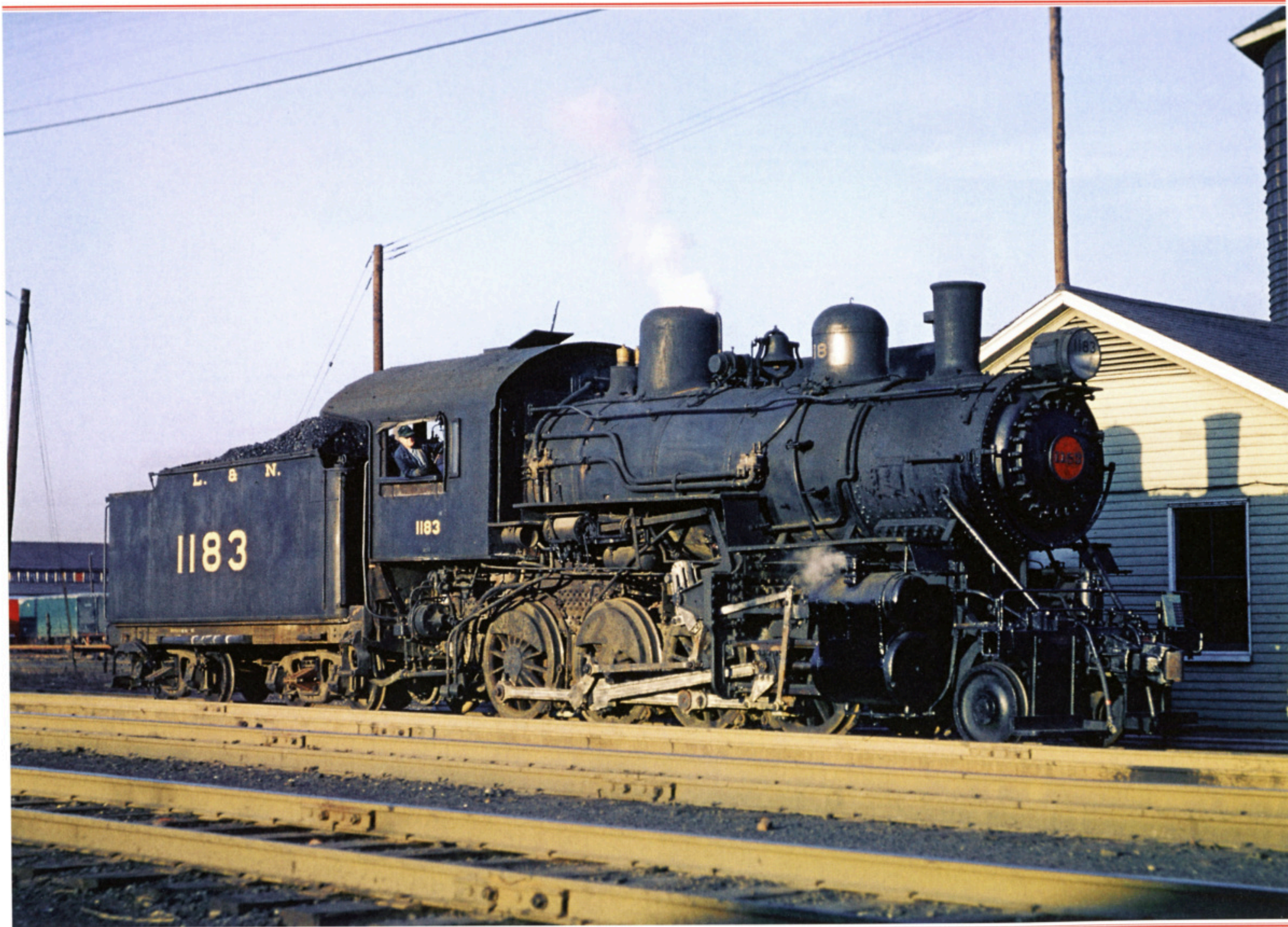
H-25B Consolidation 1183 is shown at the South Louisville shops in this scene from 1951. The 1907 Rogers engine has just completed its run through the shops, as evidenced by the fresh coat of paint on the cylinders. No doubt this visit was dedicated to running gear work. The metal board affixed to the top left of the hand rail on the pilot accompanied engines as they moved through the shop, with each craft signing off on particular work as it was completed. — Jack Fravert photo
