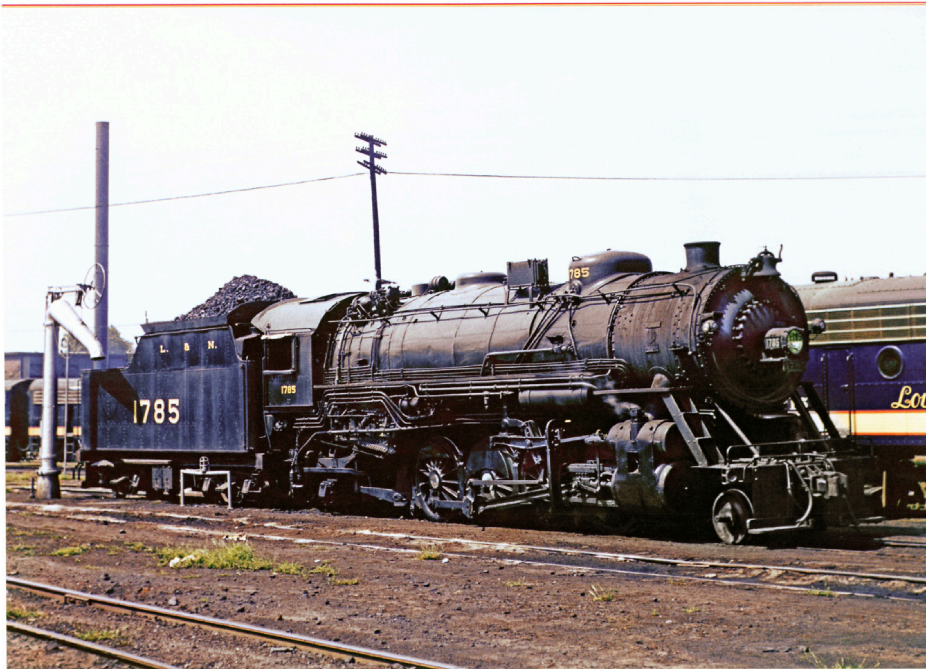
J4 number 1785 was assigned to the Knoxville & Atlanta Division for many years, as evidenced by the Automatic Train Control box and associated wiring. The train control system was used between Corbin and Etowah. While the engine appears to have been shopped recently, the internal combustion power in the background — both FP7s (right) and F7s (left) — will soon take over long before it's ready for the next rebuild that will never come. With her services no longer needed, the 1785 will be retired in August 1953. This scene was taken at South Louisville about 1952. — Jack Fravert photo
