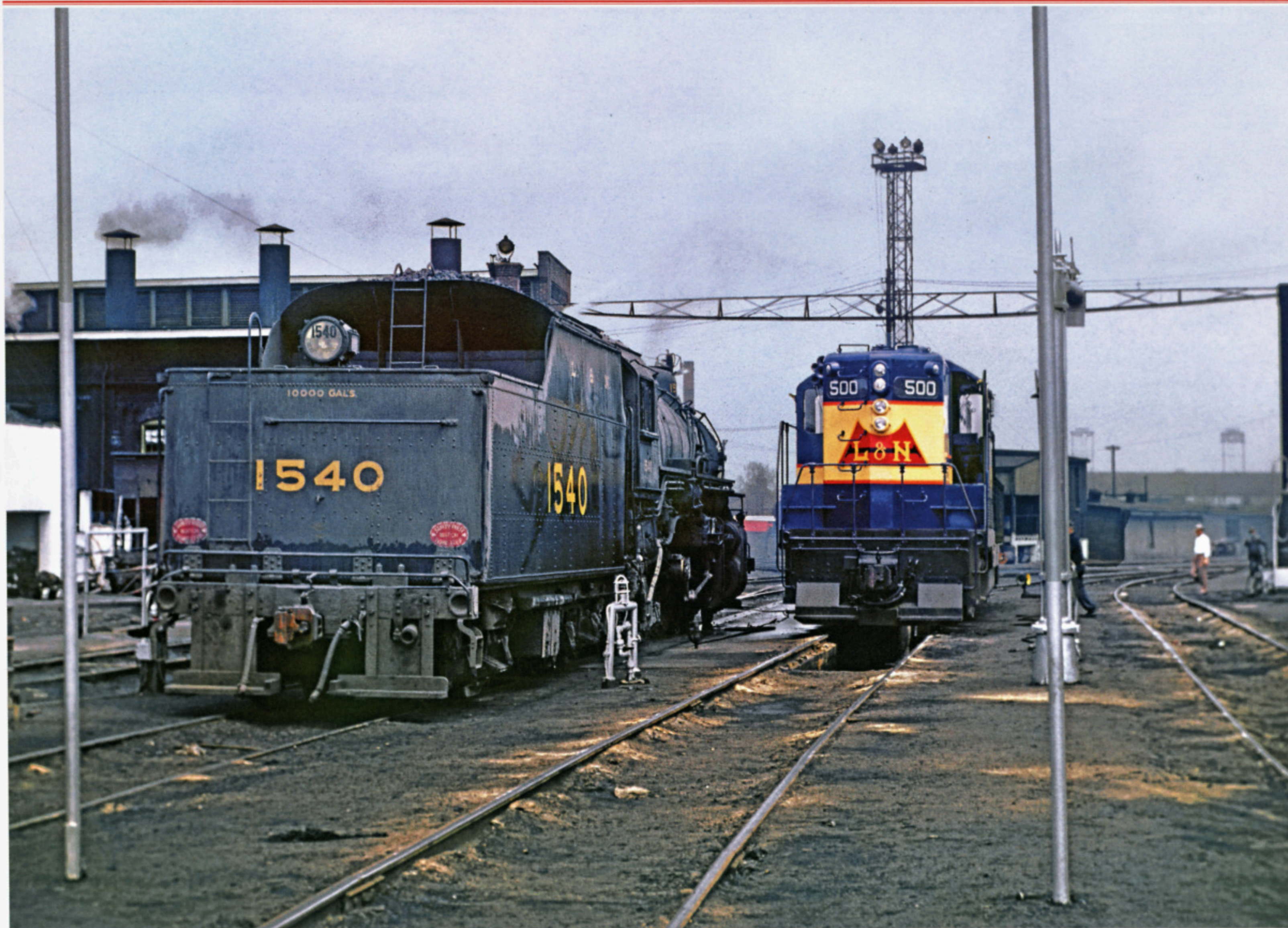
L&N In April 1951, brand-new GP7 number 500 is shown at South Louisville's roundhouse. The pretty blue-and-cream unit is the first of several dual-service units equipped with a steam generator and air signal lines for passenger service. On the adjacent track is J-3 class Mike number 1540. The short pipes protruding from the upper left of the right rear footboard is the connection for an auxiliary water tender—an increasingly common appendage for steam to increase an engine's operating range, and also minimize delays en route. After some renumberings, the GP7 was rebuilt in SCL's shops in Tampa in October 1982—becoming the first unit to be lettered "Seaboard System." — Jack Fravert photo
