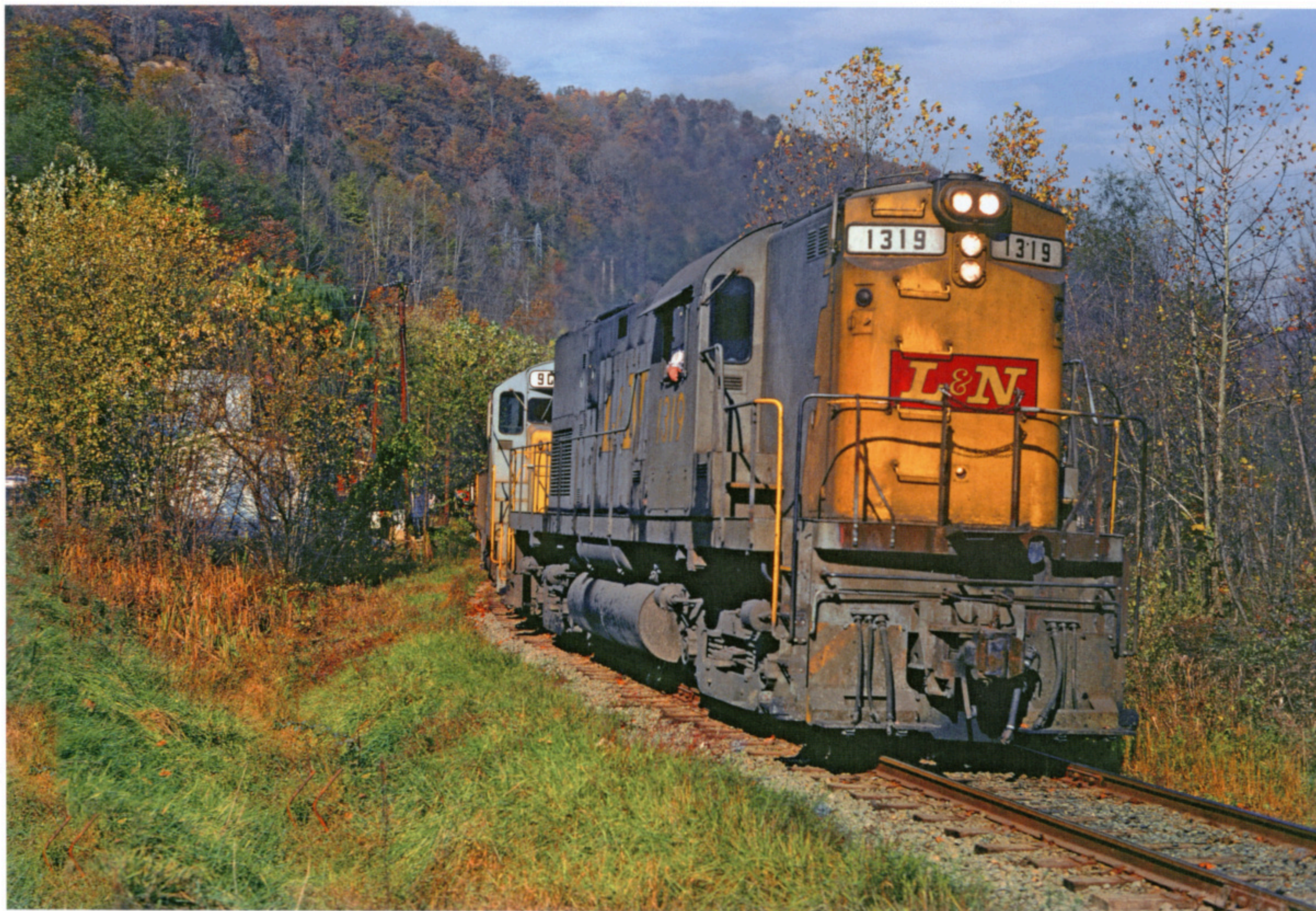
On October 25, 1975, photographer Dave Lichtenberg was lucky to catch ex-Monon C420 1319 on a Pineville mine run on the Left Fork of Straight Creek (Kentucky). No. 1319 and sister unit 1318 were equipped with steam generators (hence the high hood) to handle Monon's last passenger service, the Chicago-Louisville Thoroughbred . —Dave Lichtenberg photo
