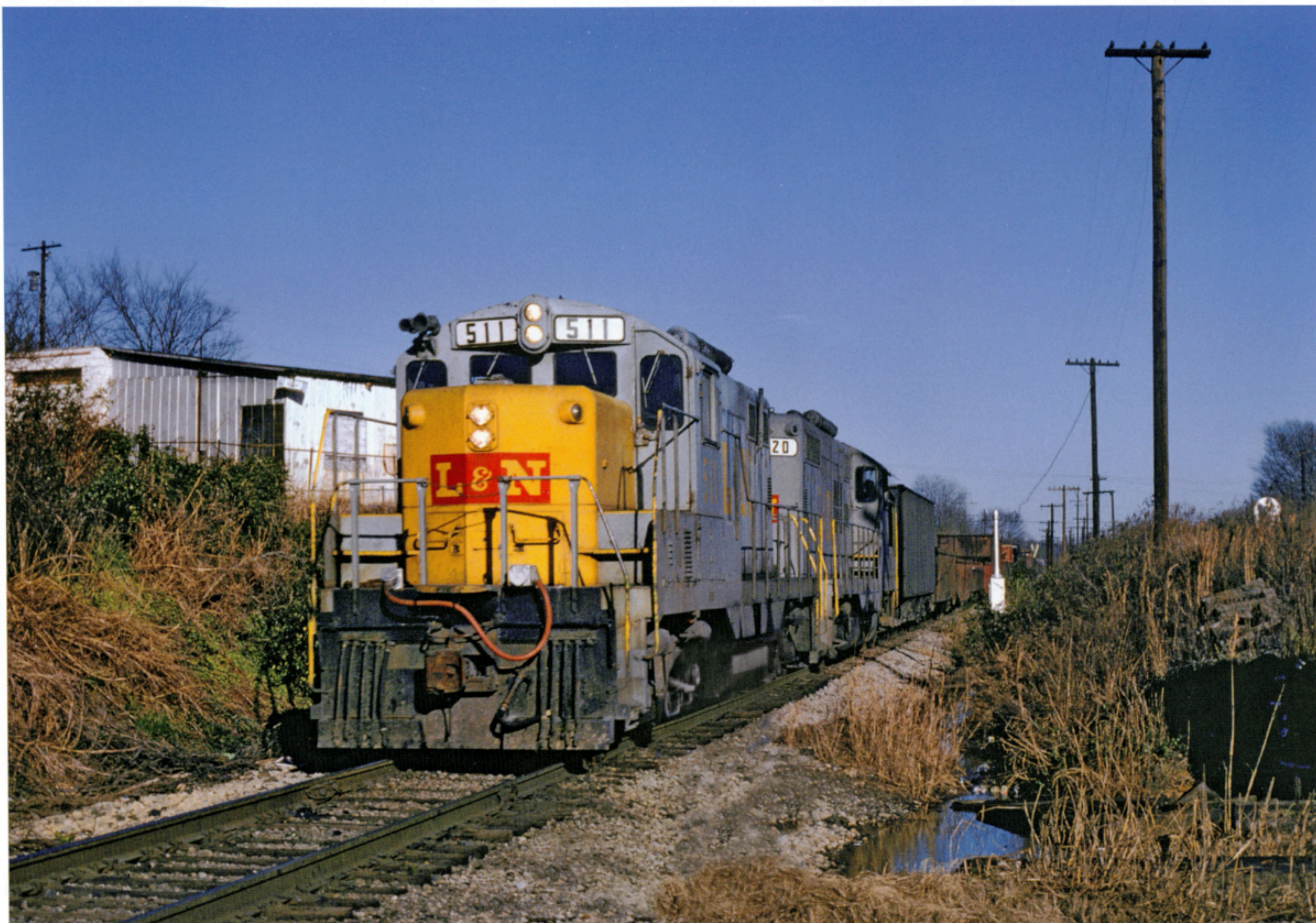
Homemade (at South Louisville) chop-nose GP9 511 is on the point of freight 571 at the 14th Street grade crossing with the Frisco at Pratt City, Alabama, on December 18, 1977. The train is running on Southern Railway trackage rights. Number 511 was rebuilt with the low nose from a dual service (freight-passenger) unit that began its career as a GP7 in 1953. It was rebuilt by EMD as a GP9 four years later after it was wrecked. — Carl Ardrey photo
