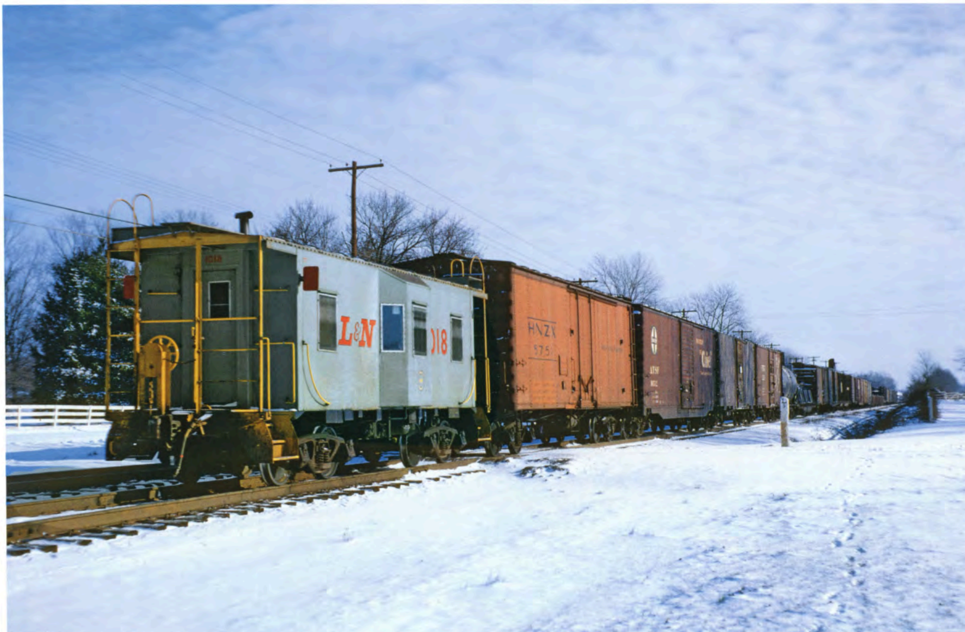
A South Louisville “shorty” steel bay window caboose brings up the rear of a “Short Line” freight at Lyndon, Kentucky. From the milepost, we know it’s nine miles to milepost 0, the bumper posts at Louisville Union Station. —Tom Smart photo
