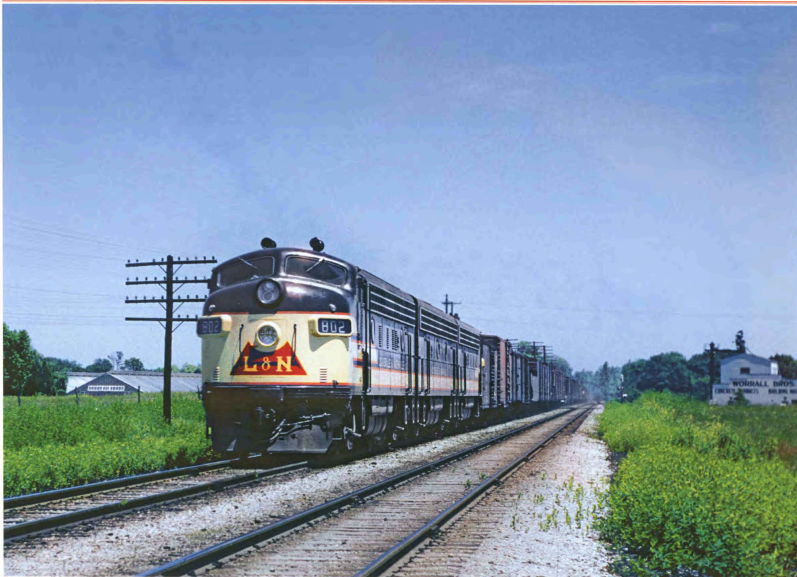
Most likely in the summer of 1950, not long after delivery, F7A Number 802 leads an A-B-A set of F-units on a southbound fast freight at North Hubbards Lane in Louisville. L&N management committed to full dieselization that year, and within the next four years, steam would be largely swept aside on such main line assignments. — Jack Fravert photo
