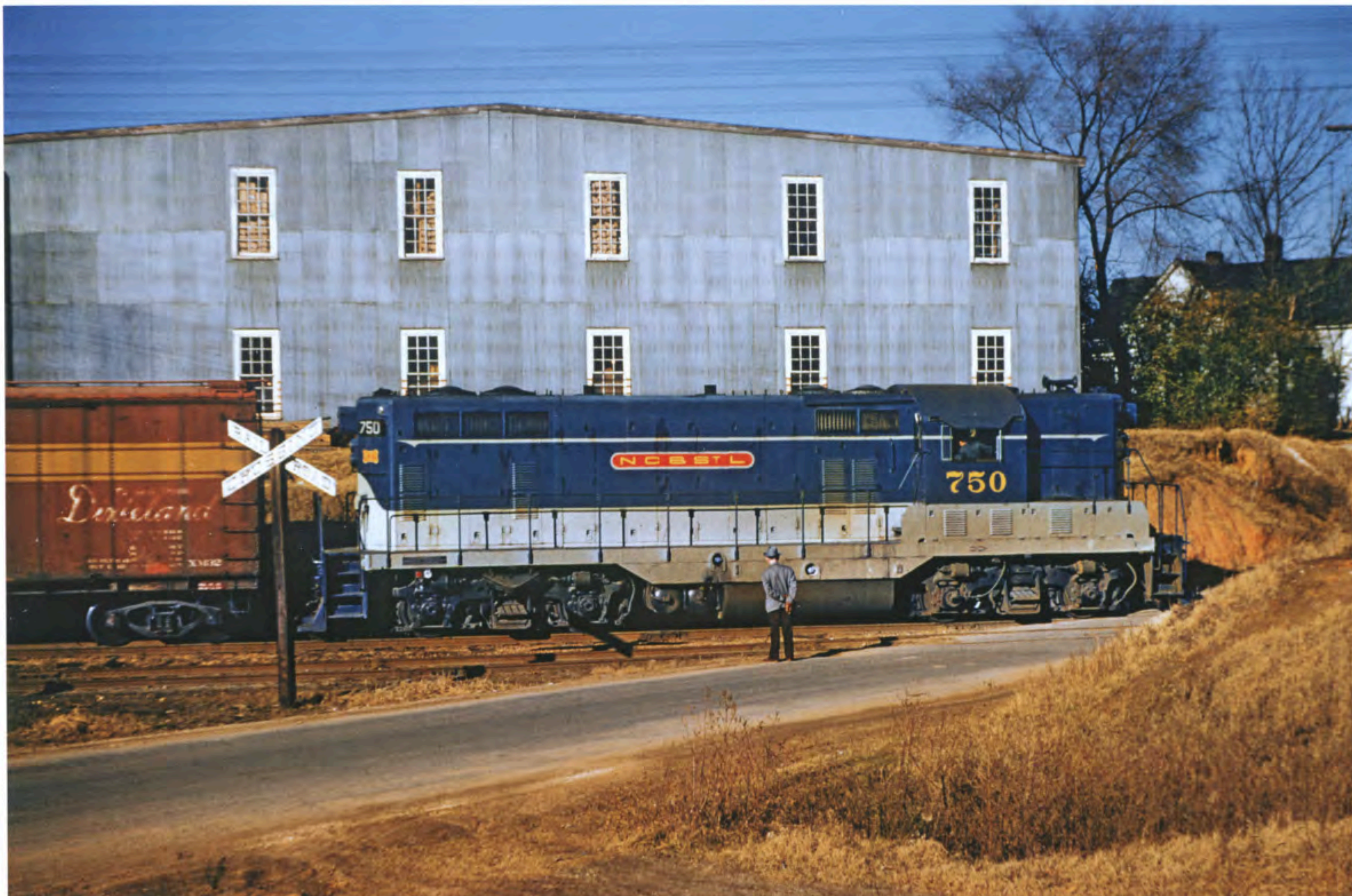
Nashville, Chattanooga & St. Louis GP7 Number 750 was one of five such units equipped with a steam generator to handle both passenger as well as freight (and, unlike freight-only units, painted blue and gray, same as the F-units). In common with similar units, the air reservoirs were later relocated to the top of the long hood allowing a larger water storage tank (from 800 to 1200 gallons). The unit is shown working a local freight in Lexington, Tennessee, on December 23, 1954. —Jim Ozment photo, Steve Forrest collection
