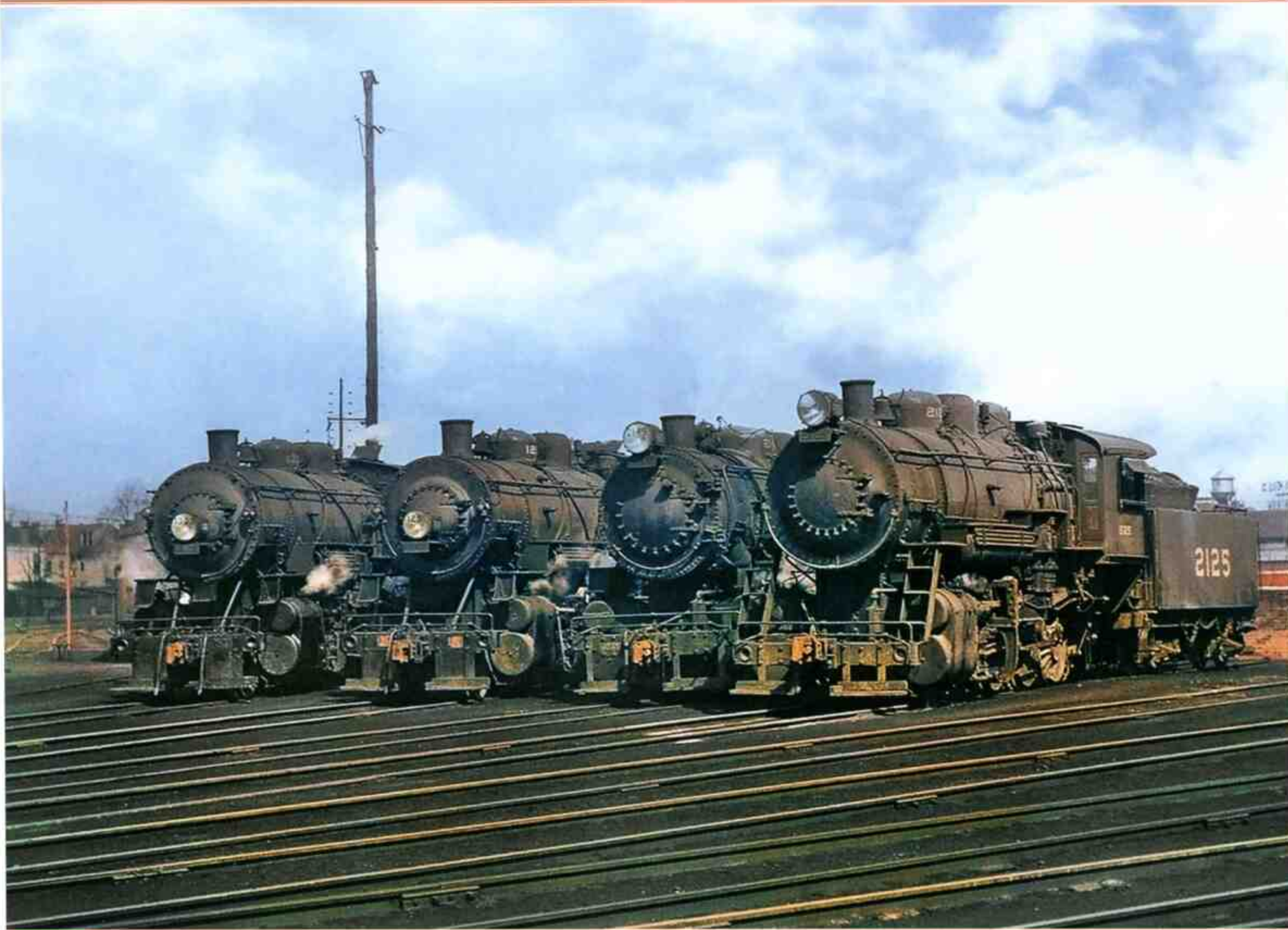
Pictured on the garden tracks at the South Louisville roundhouse, circa 1950, are four veterans from L&N's steam fleet. From left to right are 1303 and 1291 (both H28A Consolidations built at the shops) and two heavy 0-8-0 switchers. C-2 class 2149 was built by Alco, while 2125 is a C-1 built at South Louisville. — Jack Fravert photo
